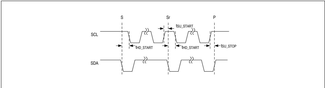
Figure 8. I<sup>2</sup>C Start Stop
