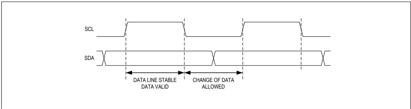
Figure 7. I<sup>2</sup>C Bit Transfer
