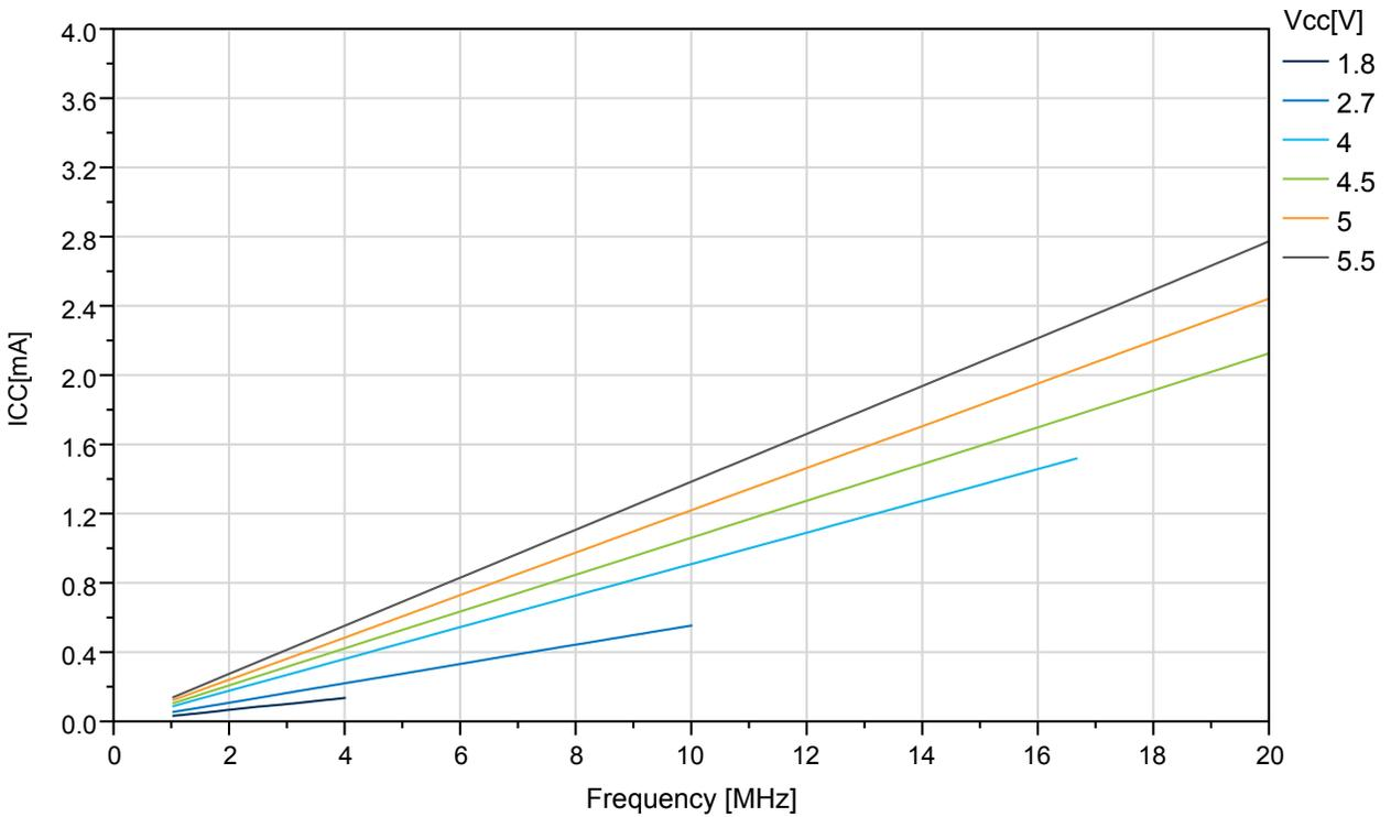
**Figure 33-54. ATmega324PB: Reset Supply Current vs.  $V_{CC}$  (Excluding current through Reset Pullup)**
