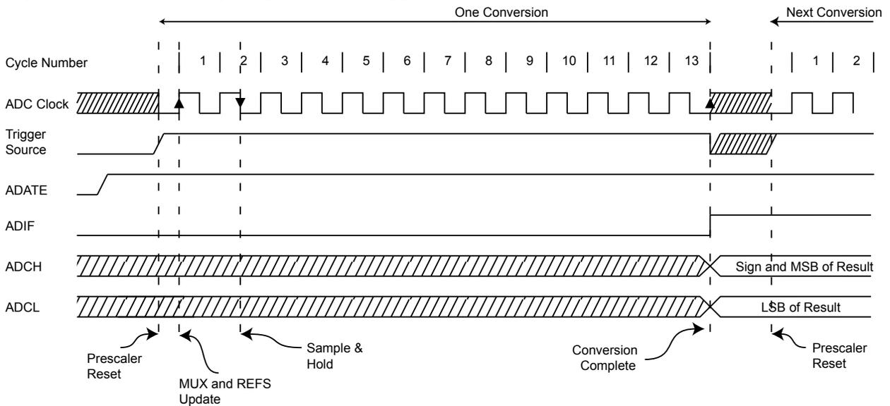
Figure 27-7. ADC Timing Diagram, Free Running Conversion
