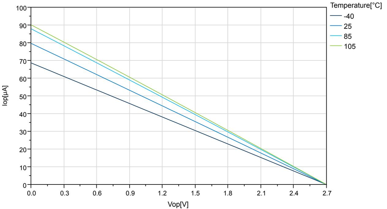
**Figure 33-18. ATmega324PB: I/O Pin Pull-up Resistor Current vs. Input Voltage ( $V_{CC} = 5V$ )**
