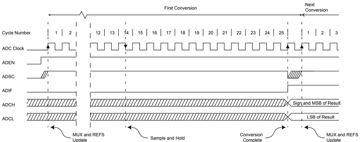
Figure 27-5. ADC Timing Diagram, Single Conversion
