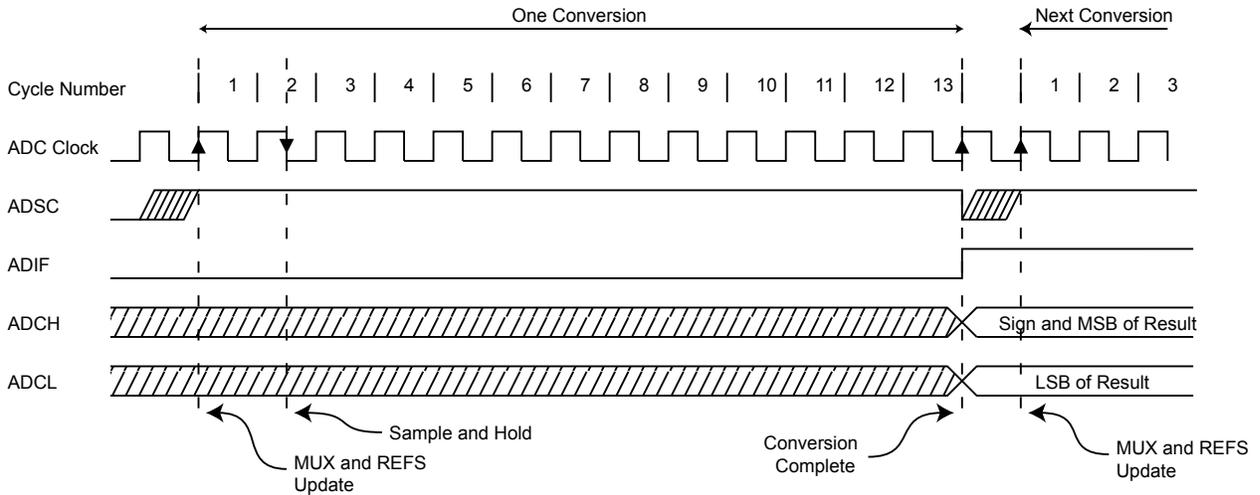
Figure 27-6. ADC Timing Diagram, Auto Triggered Conversion
