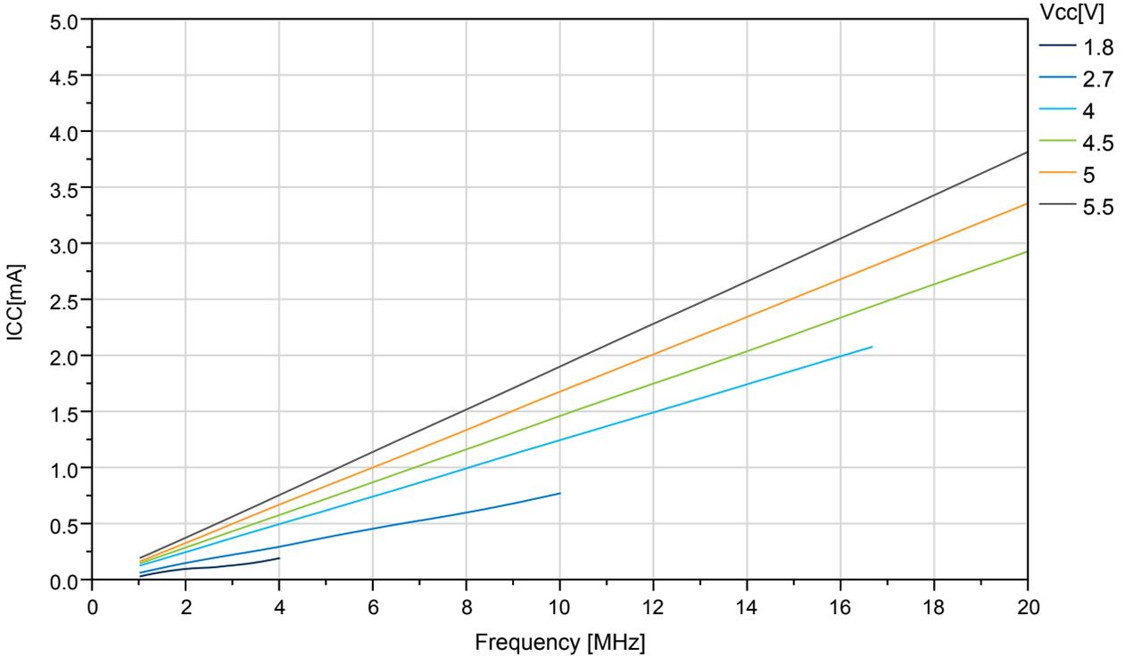
**Figure 33-10. ATmega324PB: Idle Supply Current vs.  $V_{CC}$  (Internal RC Oscillator, 128kHz)**
