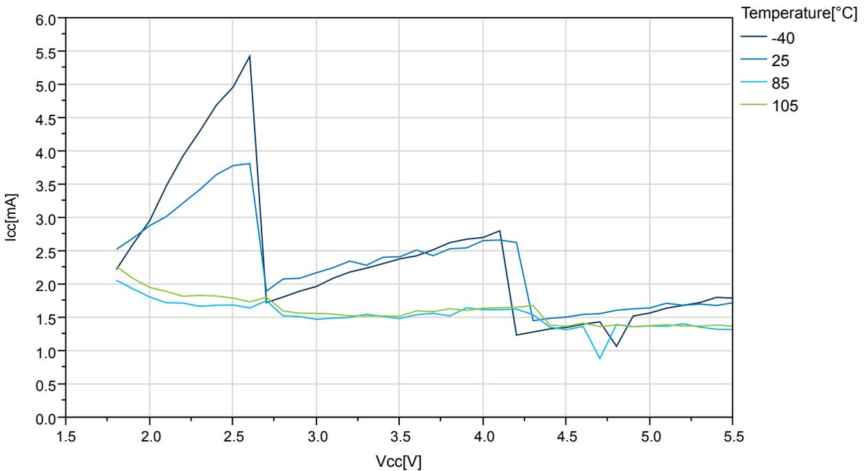
33.12 Current Consumption in Reset and Reset Pulse Width
