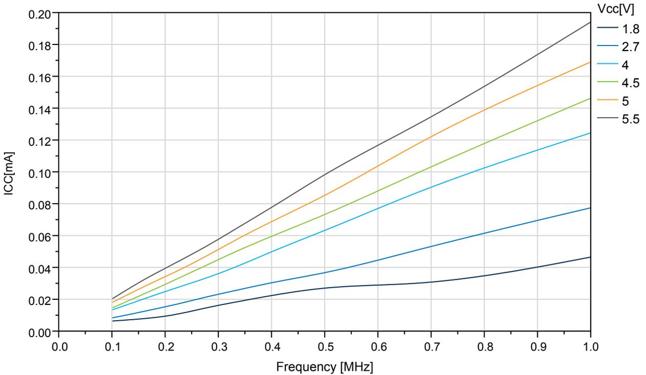
Figure 33-9. ATmega324PB: Idle Supply Current vs. Frequency (1-20MHz)
