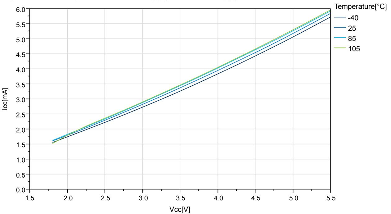
**Figure 33-6. ATmega324PB: Active Supply Current vs. VCC (With ADC, Conversion 50kHz)**
