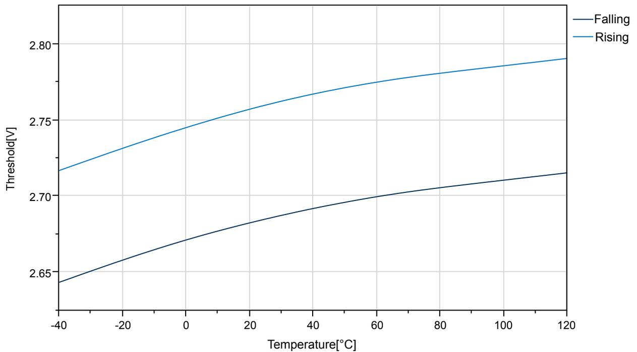
**Figure 33-34. ATmega324PB: BOD Thresholds vs. Temperature (BODLEVEL is 4.3V)**
