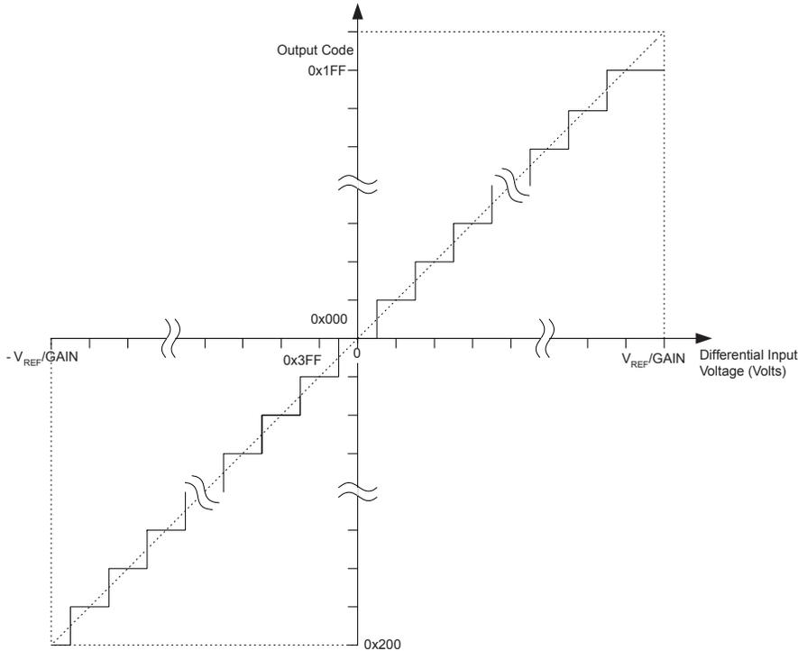
The table below shows the resulting output codes if the differential input channel pair (ADC<sub>n</sub> - ADC<sub>m</sub>) is selected with a gain of GAIN and a reference voltage of V<sub>REF</sub>.
