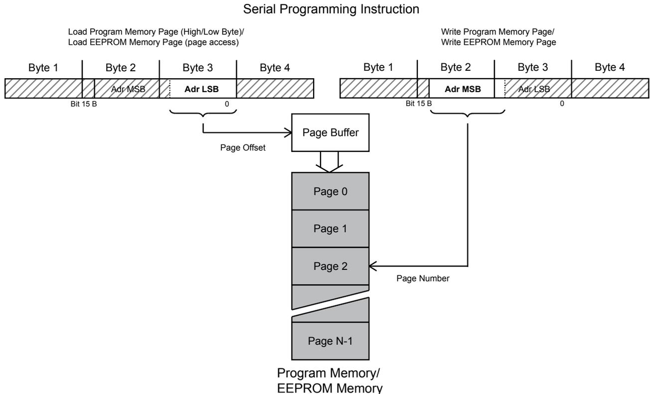
31.9.4 SPI Serial Programming Characteristics
