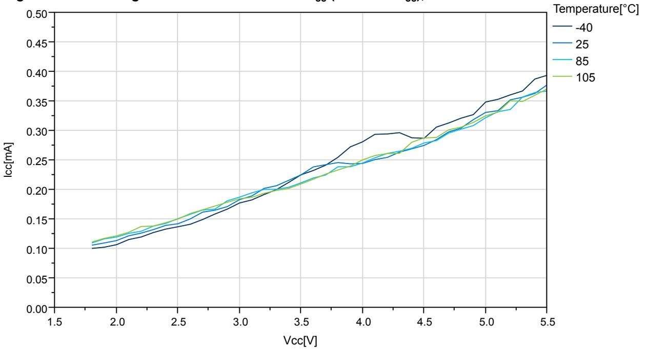
**Figure 33-49. ATmega324PB: Analog Comparator Current vs.  $V_{CC}$**
