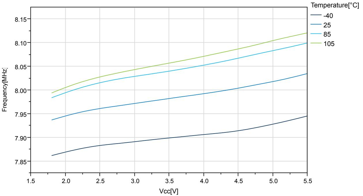
**Figure 33-44. ATmega324PB: Calibrated 8MHz RC Oscillator Frequency vs. Temperature**
