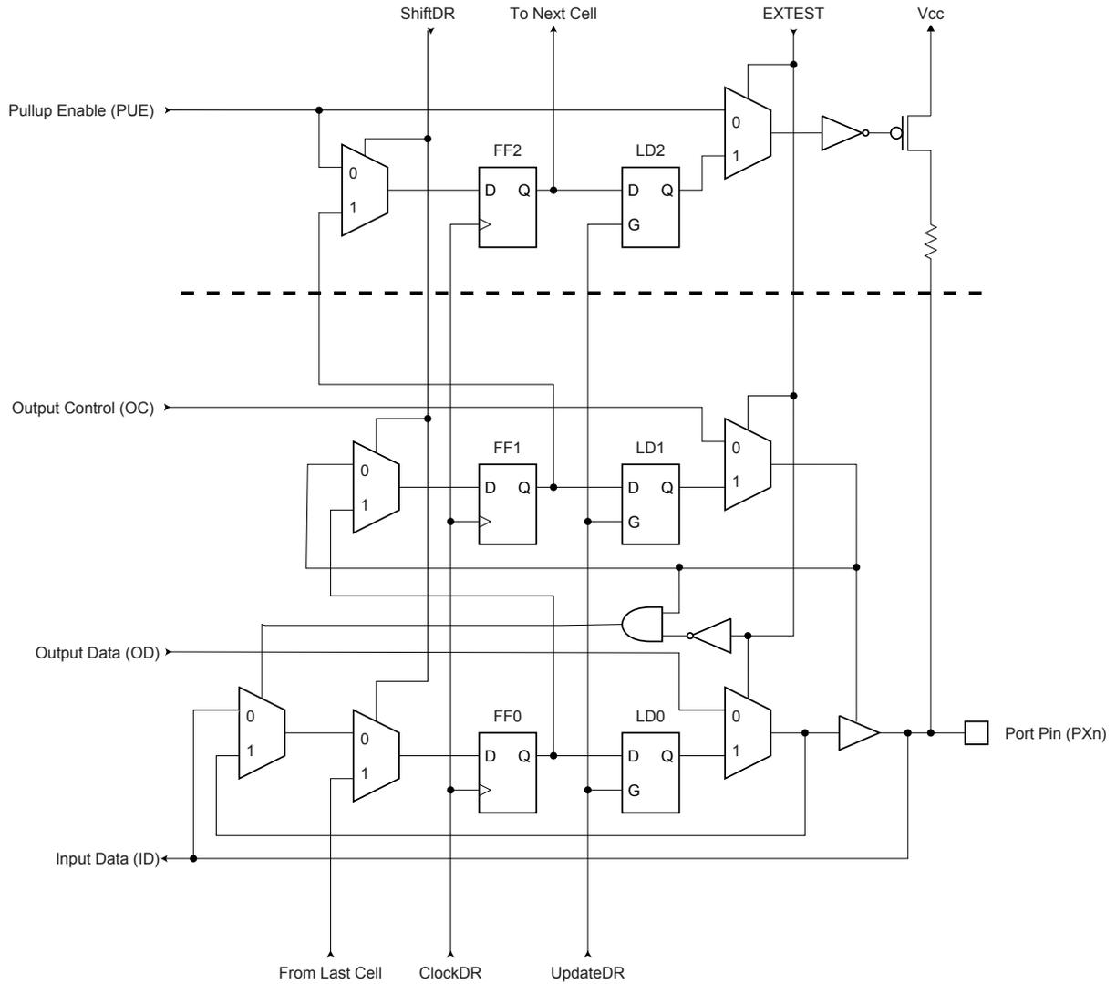
**Figure 29-6. General Port Pin Schematic diagram**
