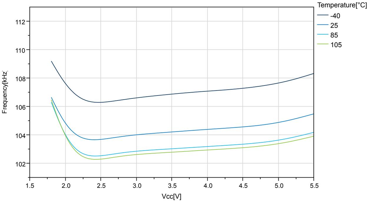
**Figure 33-43. ATmega324PB: Calibrated 8MHz RC Oscillator Frequency vs. V<sub>CC</sub>**
