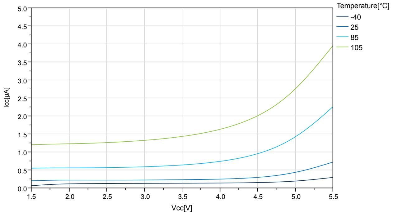
**Figure 33-14. ATmega324PB: Power-Down Supply Current vs.  $V_{CC}$  (Watchdog Timer Enabled)**
