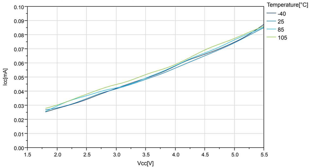
**Figure 33-4. ATmega324PB: Active Supply Current vs.  $V_{CC}$  (Internal RC Oscillator, 1MHz)**
