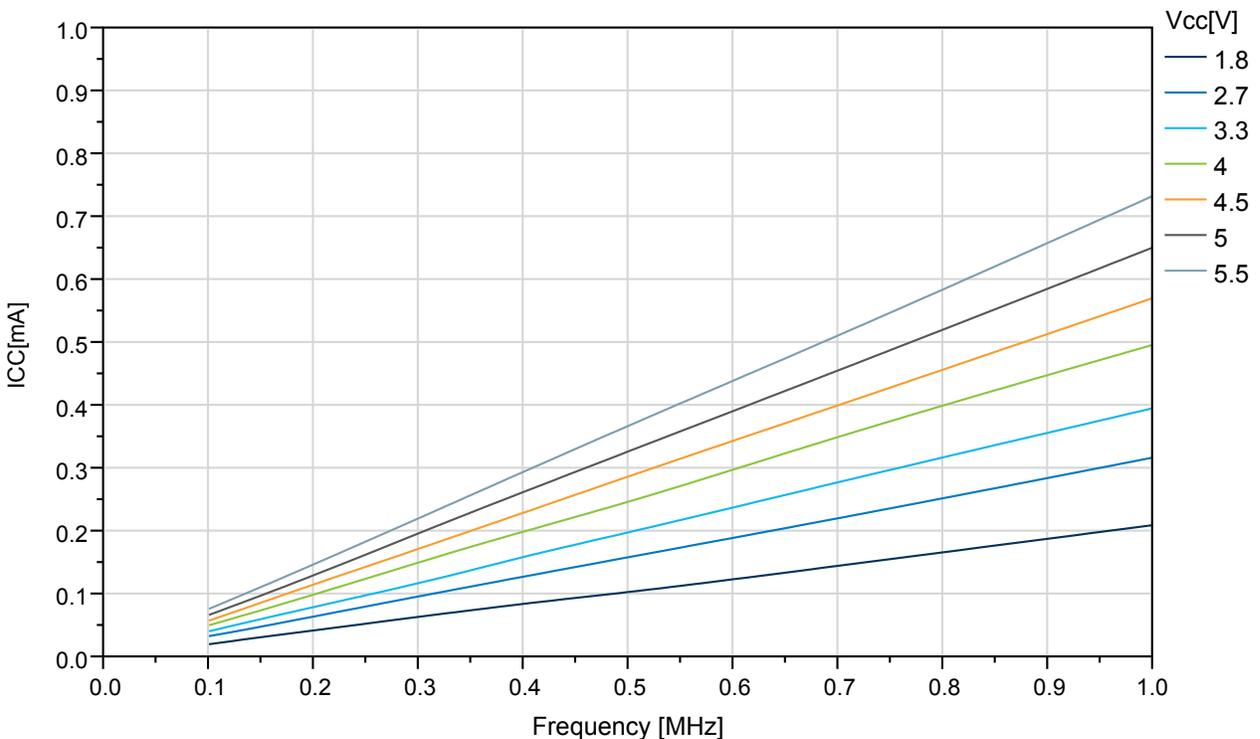
**Figure 33-2. ATmega324PB: Active Supply Current vs. Frequency (1-20MHz)**
