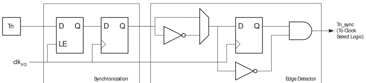
The synchronization and edge detector logic introduces a delay of 2.5 to 3.5 system clock cycles from an edge has been applied to the T1/T0 pin to the counter is updated.
