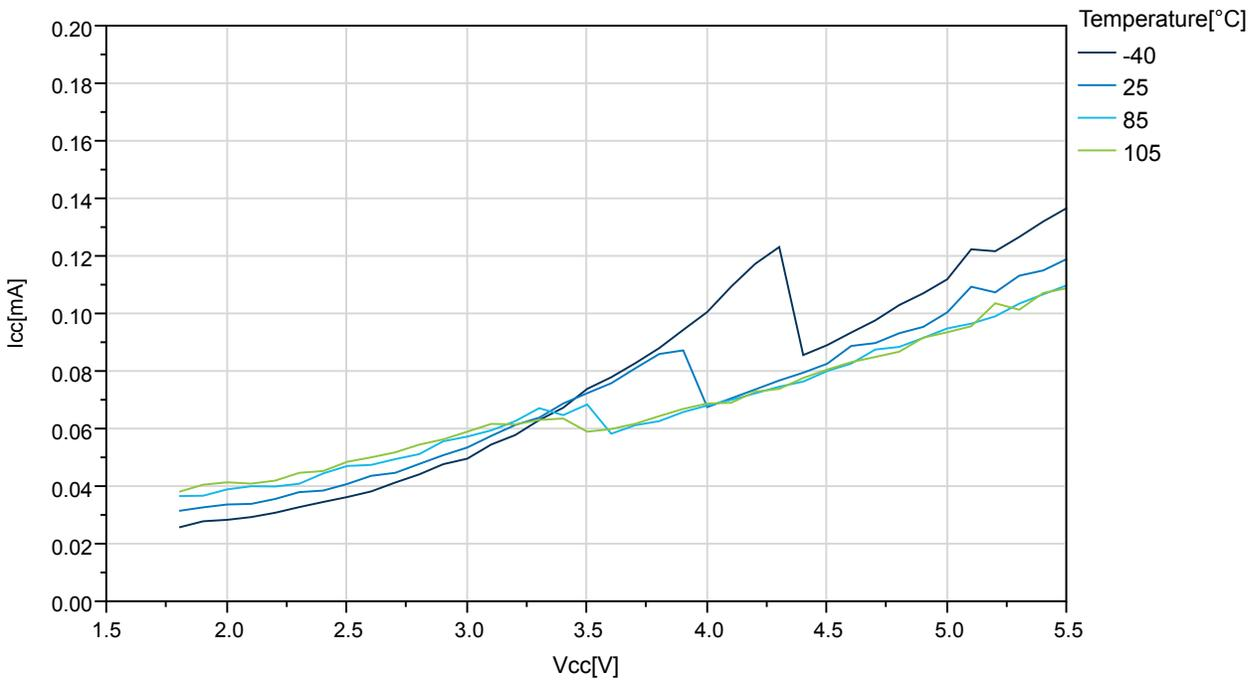
**Figure 33-50. ATmega324PB: AREF External Reference Current vs.  $V_{CC}$**
