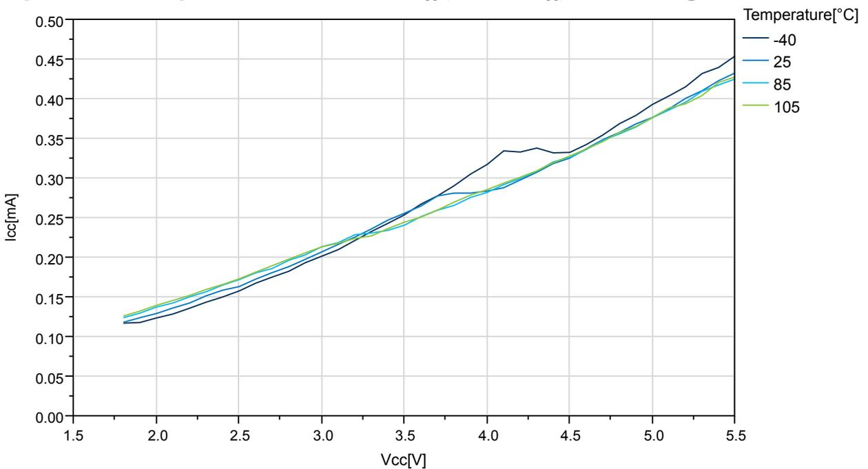
**Figure 33-48. ATmega324PB: ADC Current vs.  $V_{CC}$  ( $AREF = AV_{CC}$ ), No Conversion**
