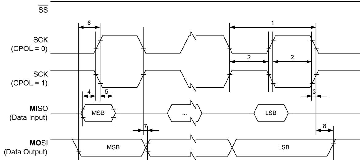
Figure 32-4. SPI Interface Timing Requirements (Slave Mode)
