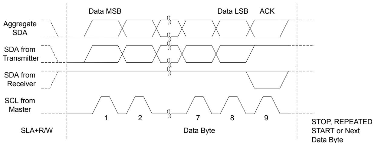
25.3.5 Combining Address and Data Packets into a Transmission
