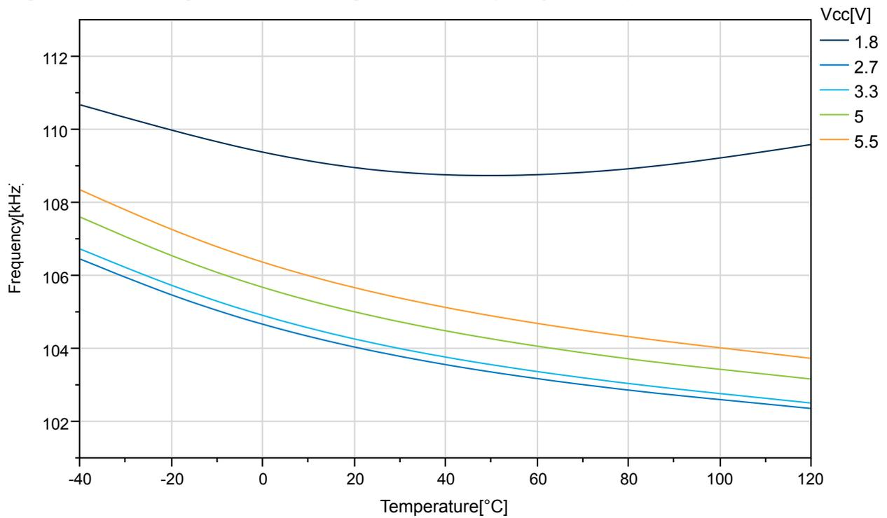
**Figure 33-42. ATmega324PB: Watchdog Oscillator Frequency vs. V<sub>CC</sub>**
