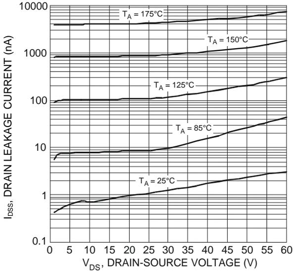
Figure 9 Typical Drain-Source Leakage Current vs. Voltage
