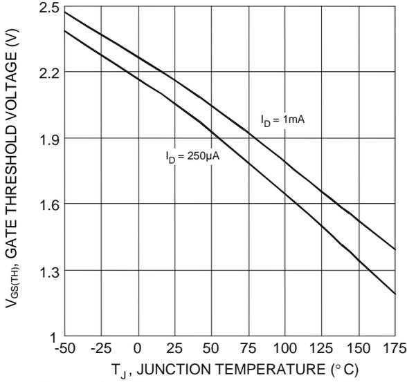
Figure 7 Gate Threshold Variation vs. Junction Temperature
