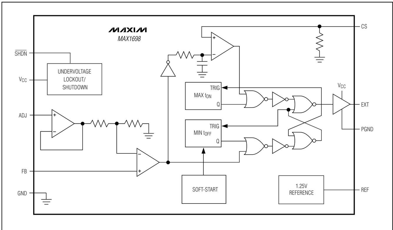
Figure 1. Functional Diagram
