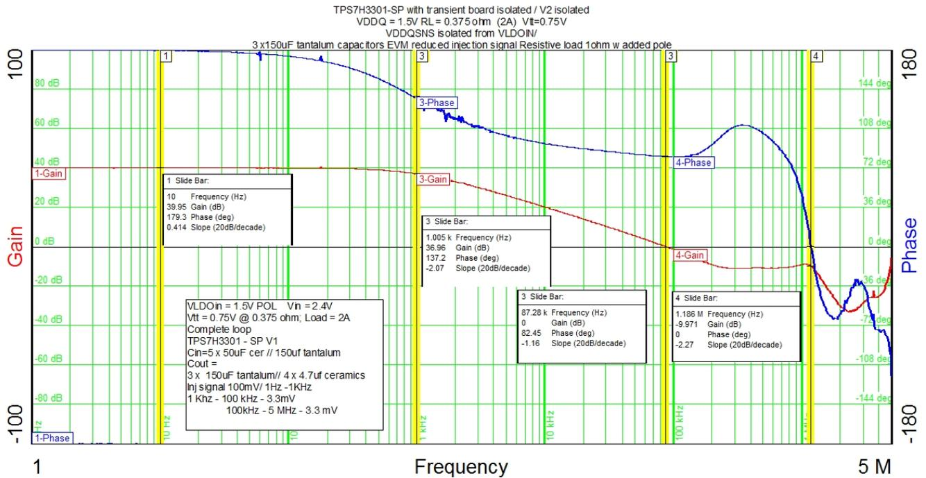
Figure 20. Bode Plot for a Typical DDR3 Configuration
