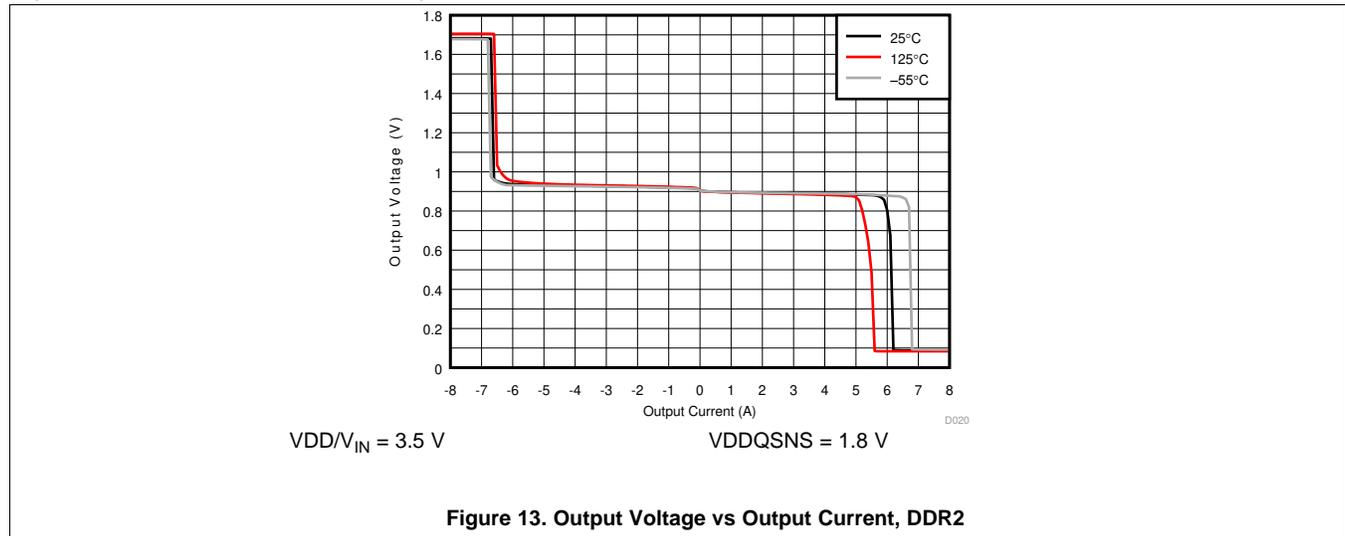
**Figure 13. Output Voltage vs Output Current, DDR2**
