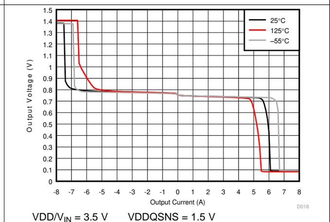
Figure 12. Output Voltage vs Output Current, DDR3
