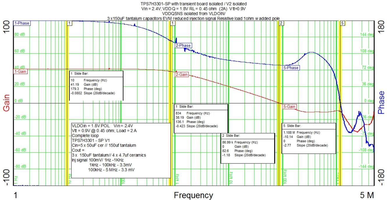
Figure 23. DDR2 2-A Load  $V_{IN} = 2.4 V$ ,  $V_{TT}/V_O = 0.9 V$
