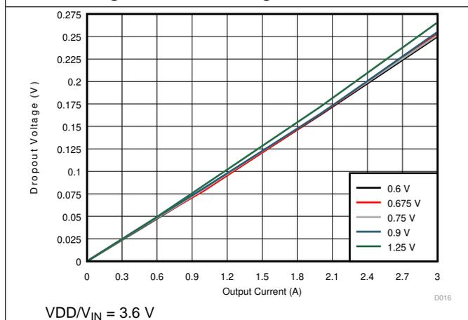
Figure 11. Dropout Voltage vs Output Current
