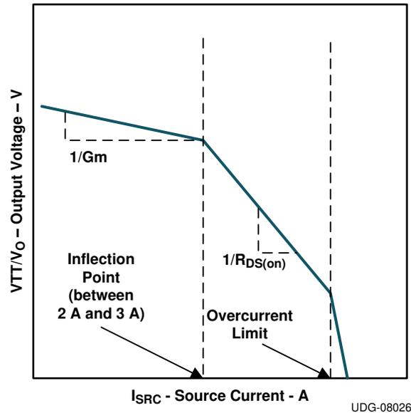
Figure 22. TPS7H3301-SP Impedance Characteristics
