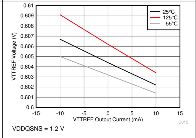
Figure 10. VTTREF Voltage vs VTTREF Current
