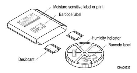
Moisture-sensitive product is packed in a dry bag containing desiccant and a humidity card according JEDEC-STD-033.
