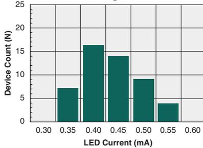
Typical  $I_F$  for Switch Dropout
