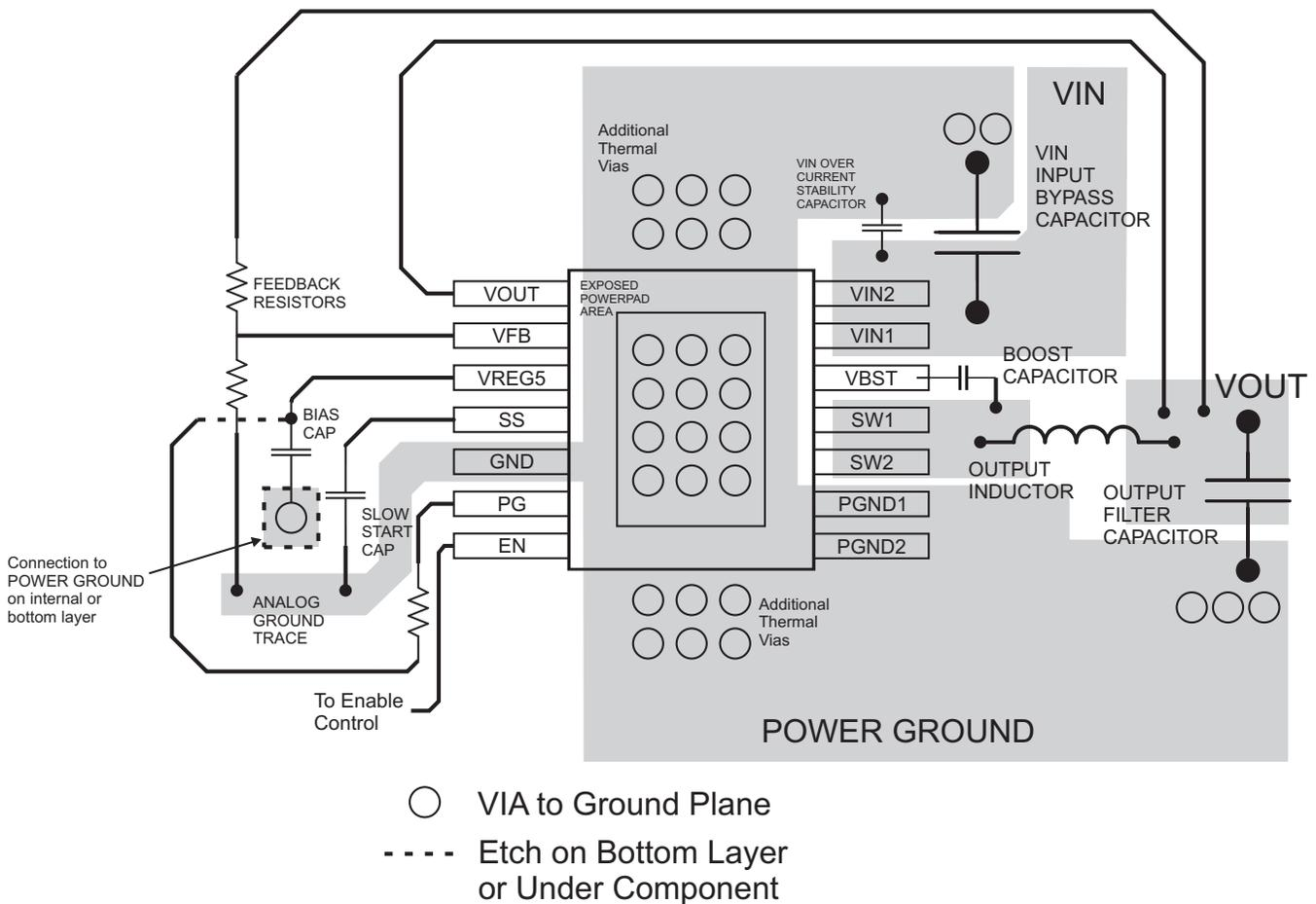
**Figure 16. PCB Layout**
