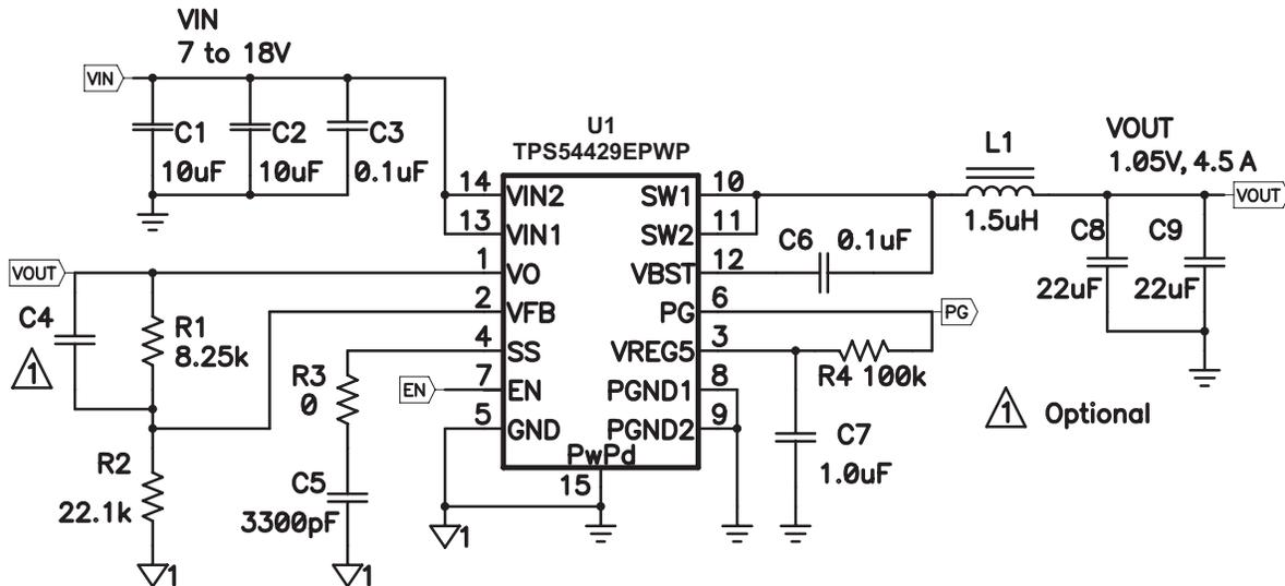
Figure 14. Schematic Diagram for This Design Example
