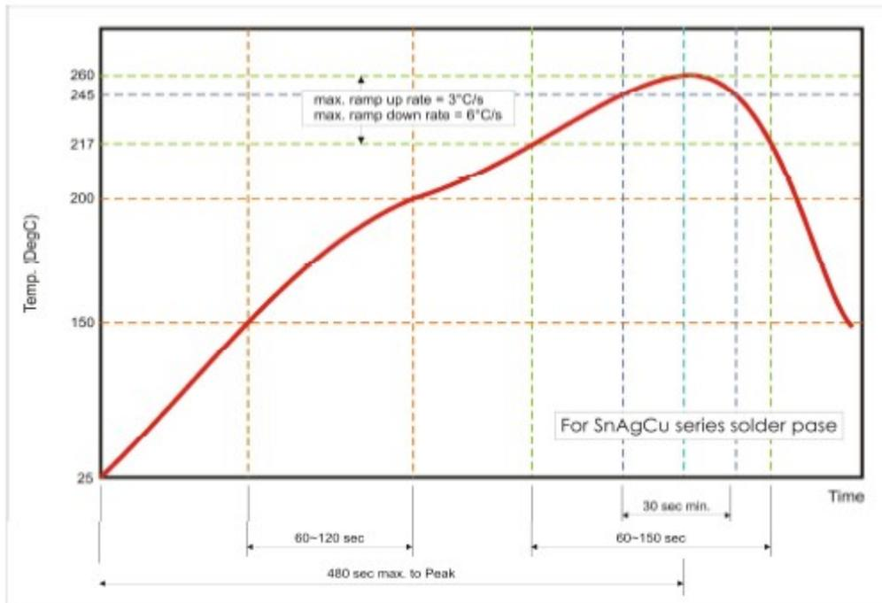
Fig 3. Infrared soldering profile for Chip Resistors WW25
