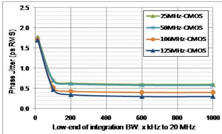
Figure 1. LVC MOS Phase Jitter (integrated phase noise)
