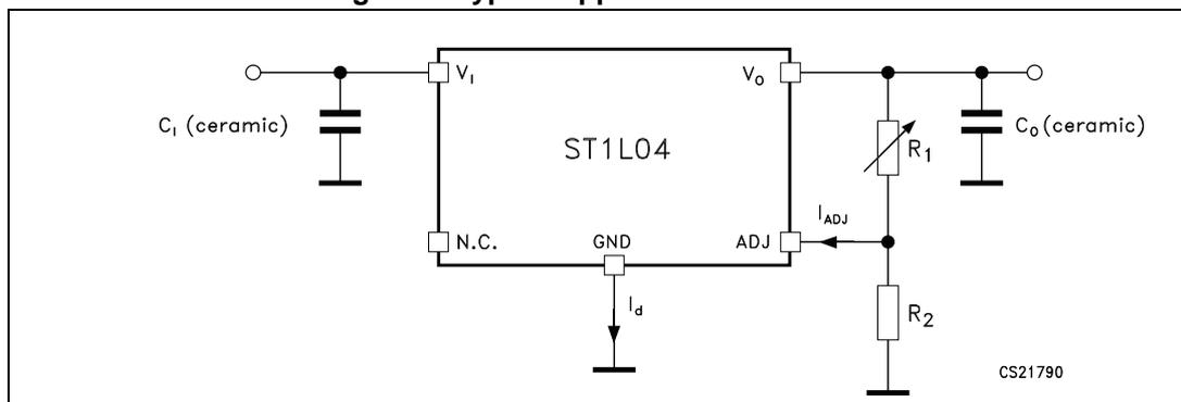
The adjustable output voltage is set by a resistor divider connected between V<sub>O</sub> and GND with its centre tap connected to ADJ. The voltage divider resistors are: R<sub>1</sub> connected between V<sub>O</sub> and ADJ and R<sub>2</sub> connected between ADJ and GND. V<sub>O</sub> is given by V<sub>REF</sub>, R<sub>1</sub>, R<sub>2</sub>, I<sub>ADJ</sub>, as follows:
