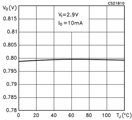
**Figure 5. Load regulation vs. temperature**
