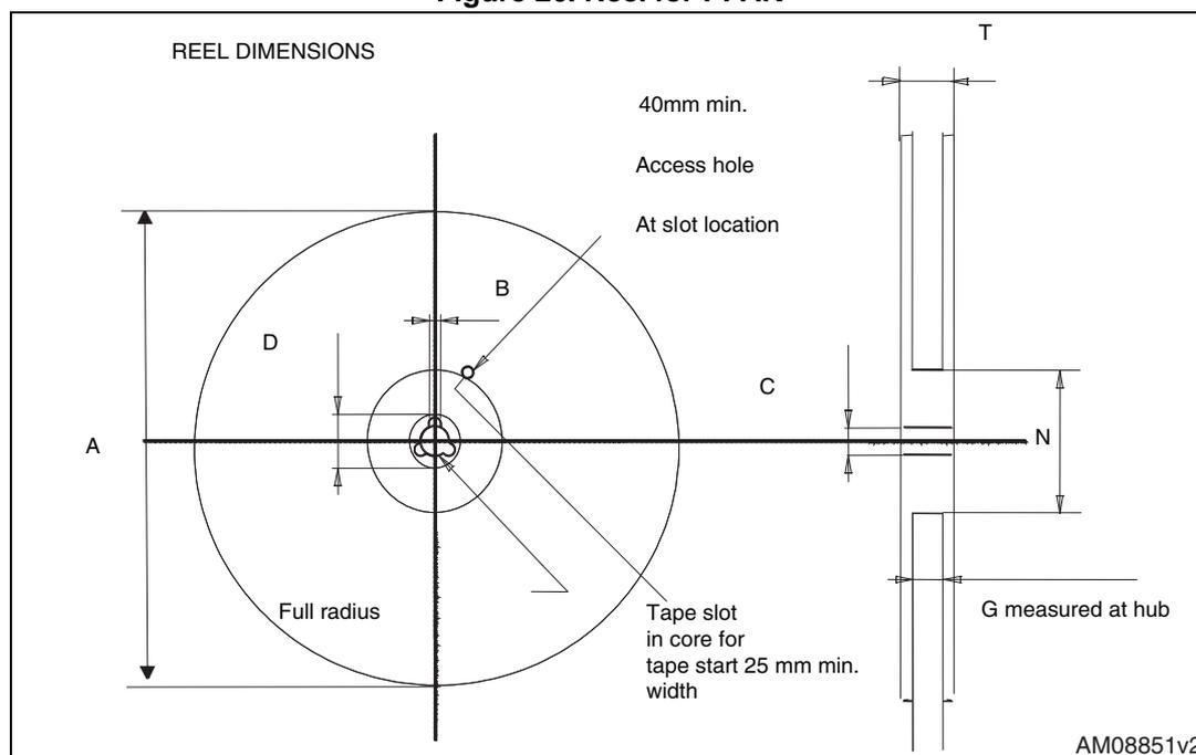
Table 7. PPAK tape and reel mechanical data
