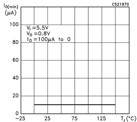
Figure 20. Adjustment current vs. temperature
