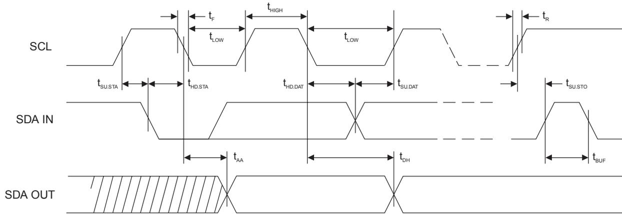
**Figure 4-2. Write Cycle Timing: SCL:**
