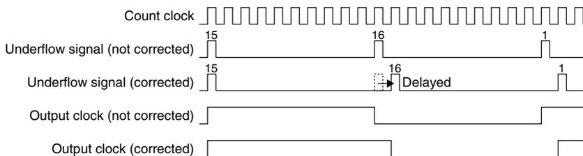
Figure 10.10.1 Delay Cycle Insertion in Fine Mode
