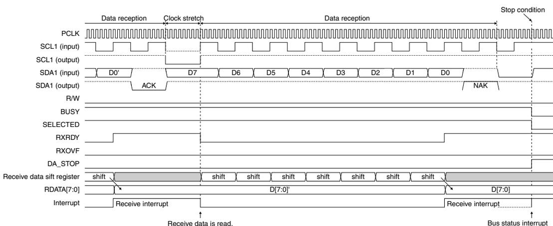
Figure 18.5.8 I2CS Timing Chart 4 (data reception → stop condition)
