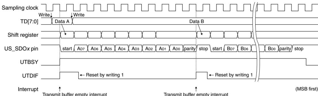
Figure 19.5.1.1 Data Transmission Timing Chart (UART mode)
