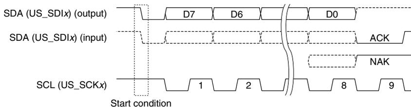
Figure 19.5.3.6 ACK and NAK
