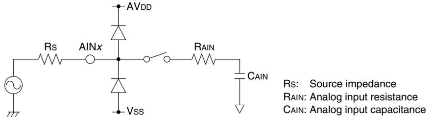
Figure 21.3.5.1 Equivalent Circuit of Analog Input Portion
