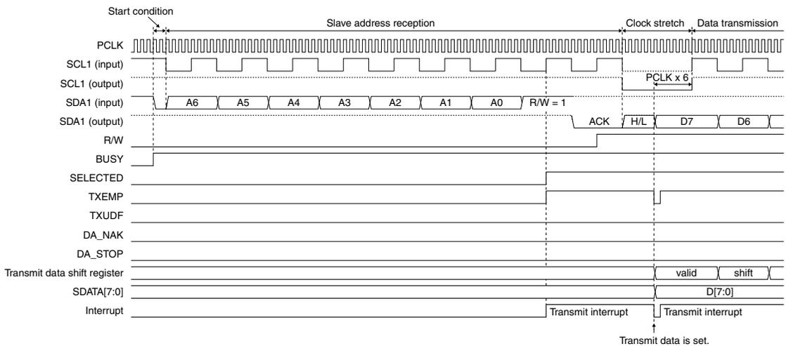
Figure 18.5.5 I2CS Timing Chart 1 (start condition → data transmission)
