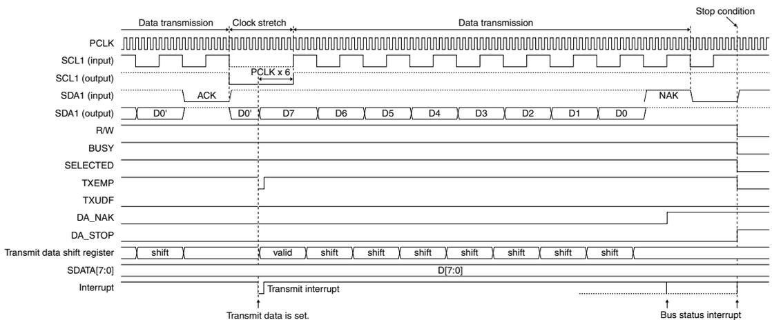
Figure 18.5.6 I2CS Timing Chart 2 (data transmission → stop condition)
