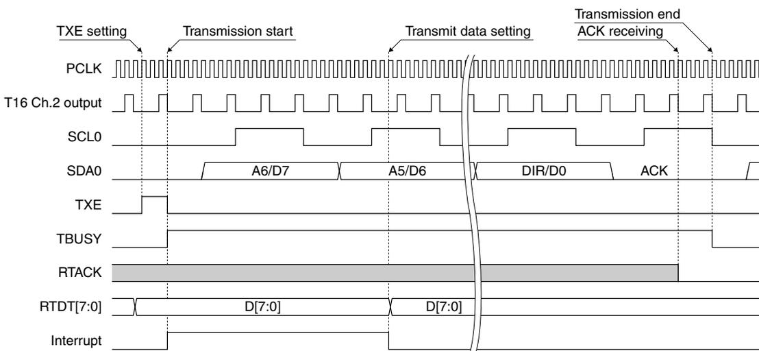
Figure 17.5.7 Slave Address Transmission/Data Transmission
