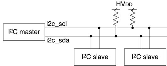
The `i2c_scl` and `i2c_sda` pins go to a low level or high impedance status when the USI module is set to I<sup>2</sup>C mode. These pins do not output a high level, so the `i2c_scl` and `i2c_sda` lines should be pulled up to `HVDD` with an external pull-up resistor.
