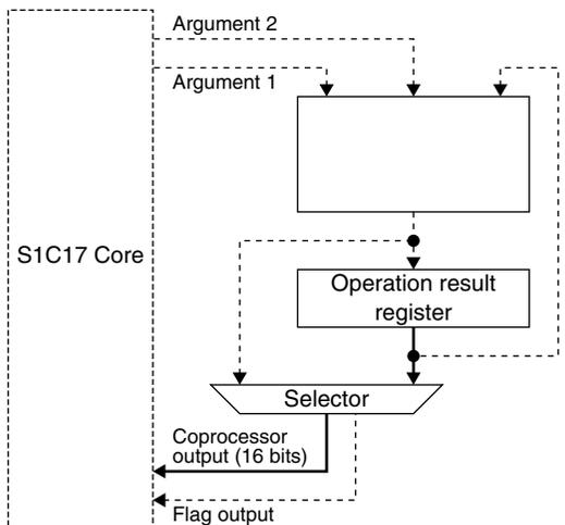
Figure 23.6.1 Data Path in Operation Result Read Mode
