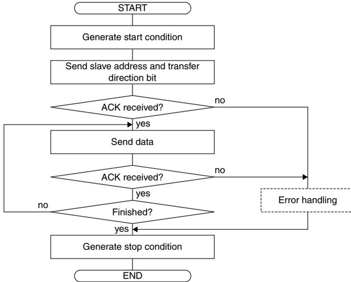
Figure 19.5.3.2 I<sup>2</sup>C Master Data Transmission Flow Chart
