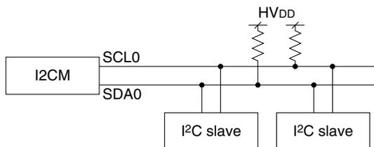
Figure 17.2.1 I<sup>2</sup>C Connection Example
