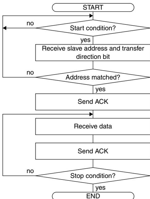
Figure 19.5.3.14 I<sup>2</sup>C Slave Data Receiving Flow Chart
