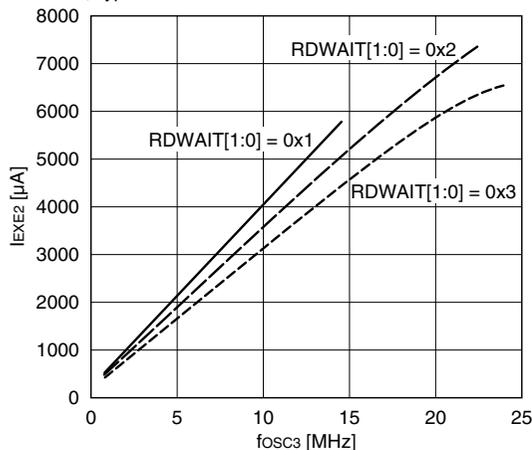
**Clock gear characteristic (OSC3 operation)**
