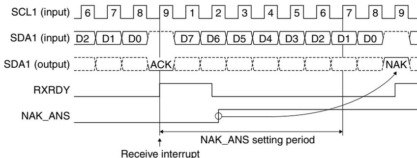
Figure 18.5.3 NAK\_ANS Setting and NAK Response Timing
