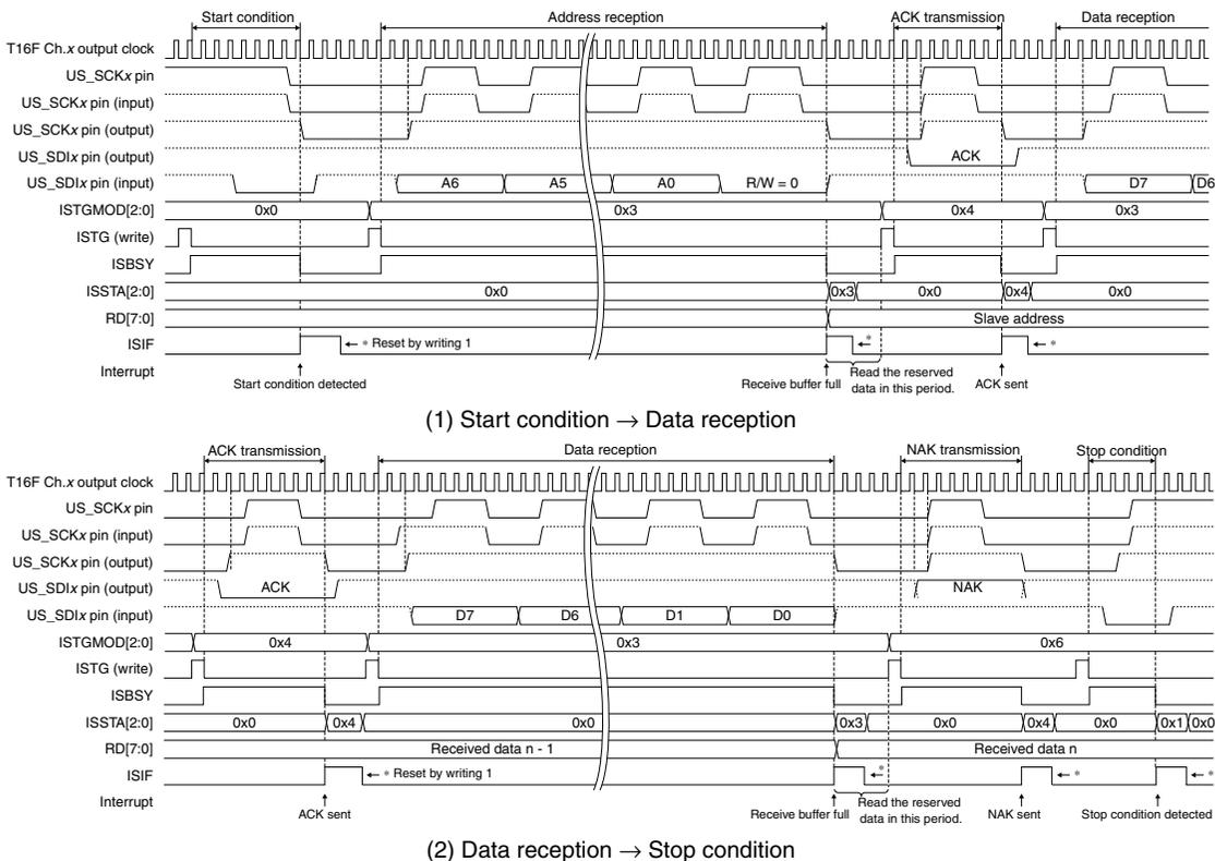
Figure 19.5.3.15 I<sup>2</sup>C Slave Data Receiving Timing Chart
