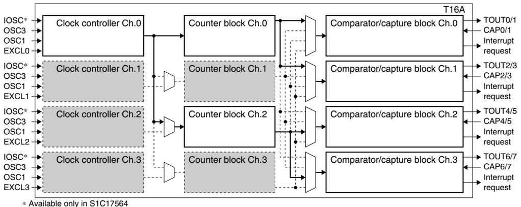
(1) Configuration Example 1 (four comparator/capture blocks × two channels)
