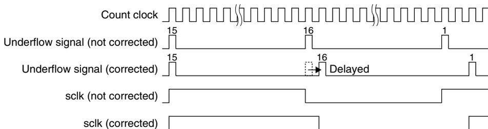
Figure 15.3.3 Delay Cycle Insertion in Fine Mode
