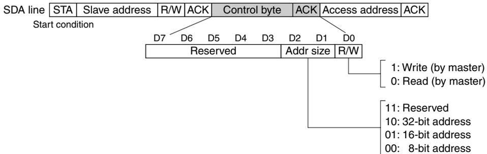
Figure 19.9.2 Control Byte Sent from I<sup>2</sup>C Master
