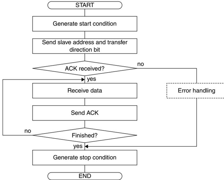
Figure 19.5.3.9 I<sup>2</sup>C Master Data Receiving Flow Chart
