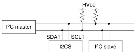
Figure 18.2.1 I<sup>2</sup>C Connection Example
