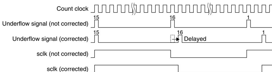
Figure 15.9.1 Delay Cycle Insertion in Fine Mode
