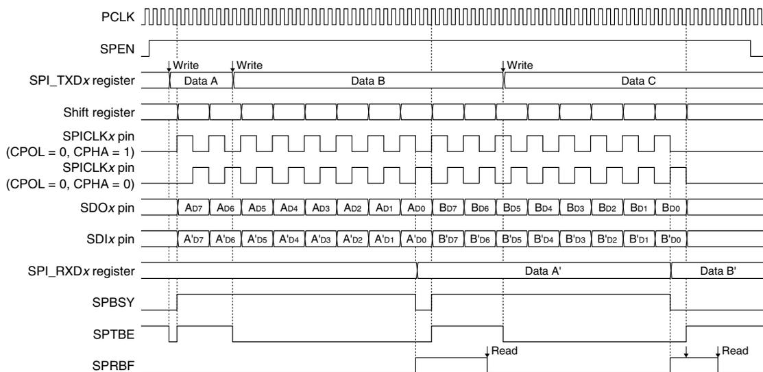
Figure 16.5.2 Data Transmission/Receiving Timing Chart (MSB first)
