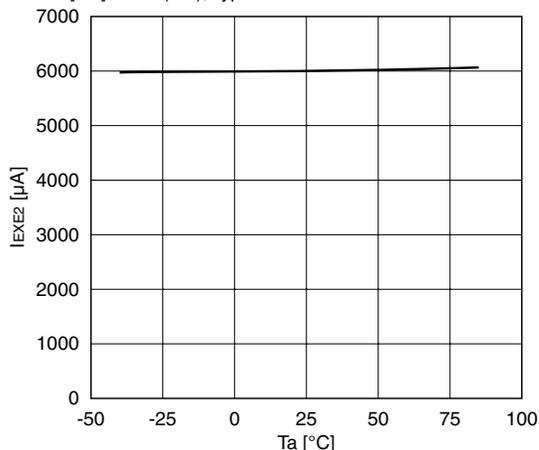
**Current consumption-temperature characteristic during execution with IOSC**
