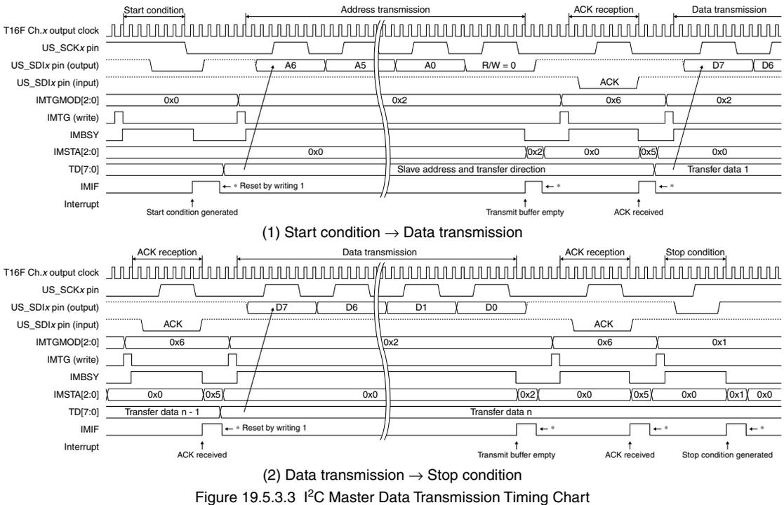
Figure 19.5.3.3 I<sup>2</sup>C Master Data Transmission Timing Chart
