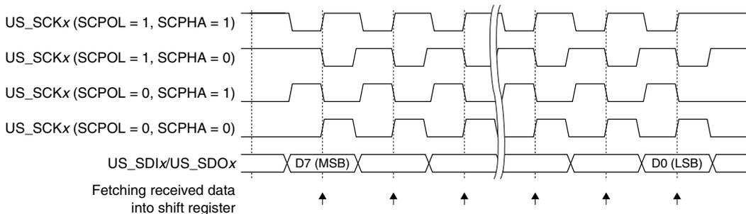
Figure 19.4.5.1 Clock and Data Transfer Timing (MSB first)
