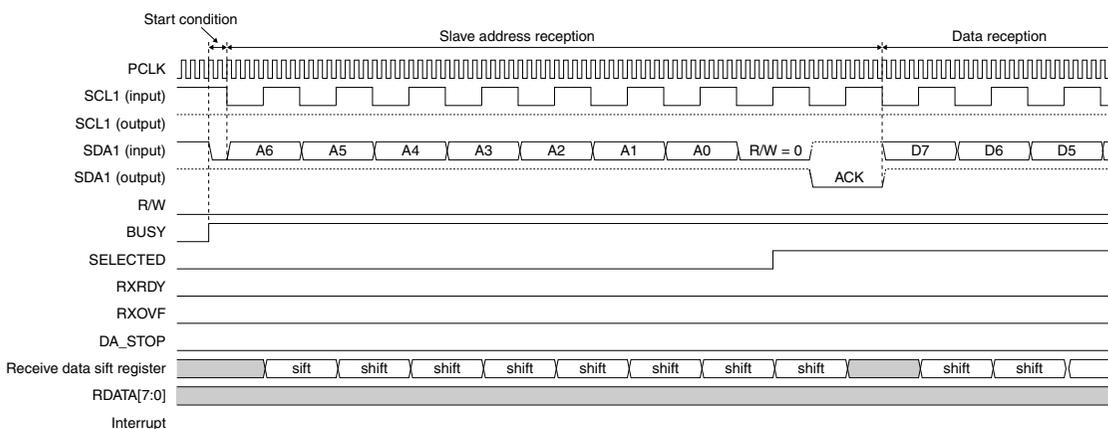
Figure 18.5.7 I2CS Timing Chart 3 (start condition → data reception)
