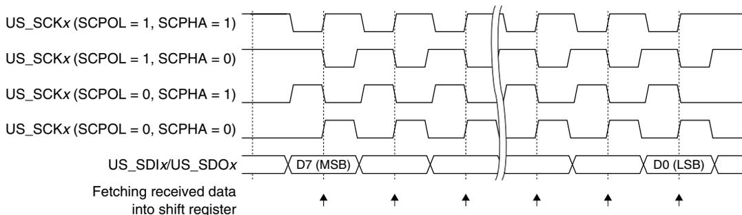
Figure 19.8.2 Clock and Data Transfer Timing
