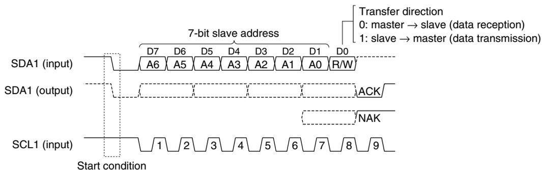
Figure 18.5.1 Receiving Slave Address and Data Direction Bit
