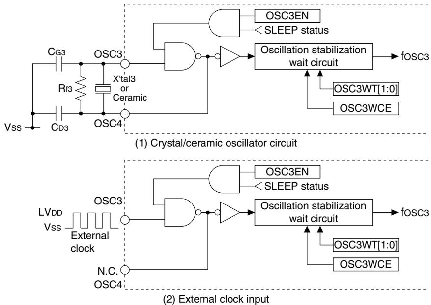
Figure 7.3.1.1 OSC3 Oscillator Circuit
