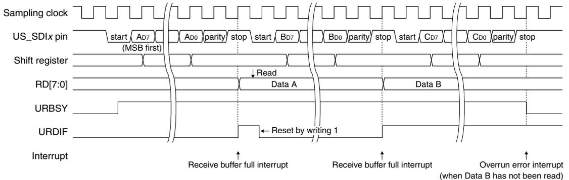
Figure 19.5.1.2 Data Receiving Timing Chart (UART mode)
