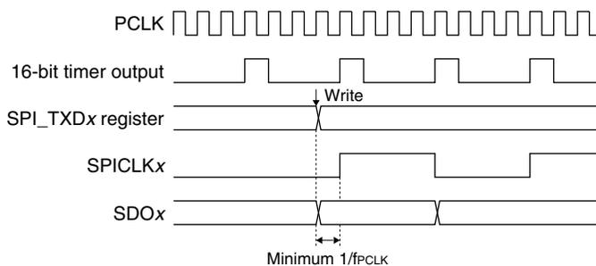
Figure 16.5.1 SDOx and SPICLKx Change Timings when CPHA = 0
