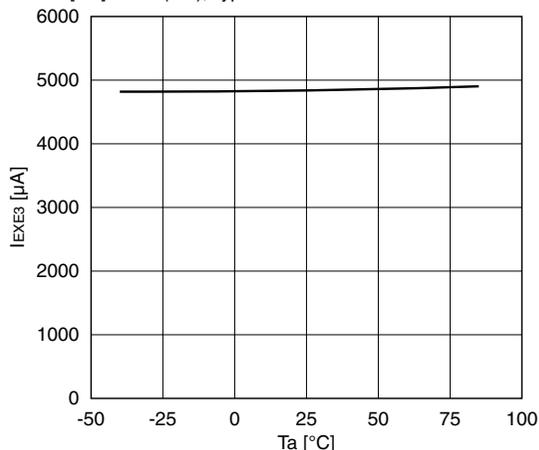
**Flash read current consumption characteristic (OSC3 operation)**
