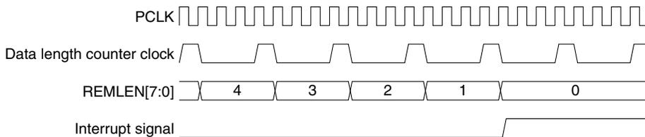
Figure 20.5.2 Underflow Interrupt Generation Timing
