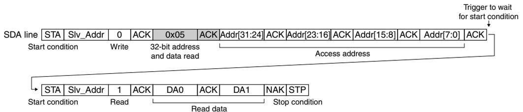
Figure 19.9.4 I<sup>2</sup>C Master Read (Data Transmission to Master)
