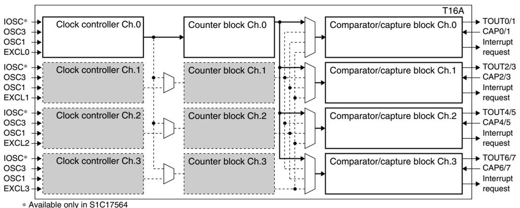
(2) Configuration Example 2 (eight comparator/capture blocks × one channel)
