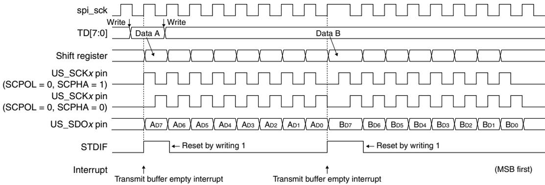
Figure 19.5.2.1 Data Transmission Timing Chart (SPI master mode)
