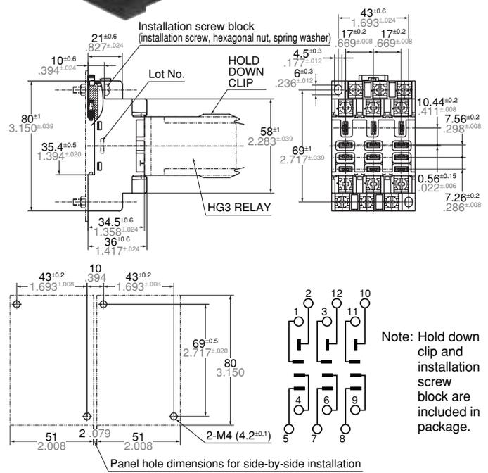
**Solder terminal socket (Hold-down clips included)**
