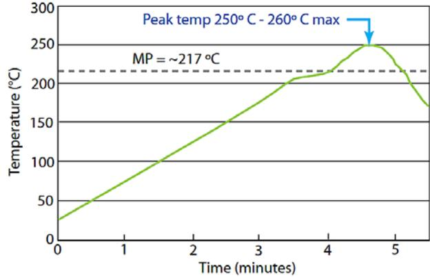
*This reflow profile is a guideline for Pb-free solder materials. Adjustments to this profile are necessary based on specific process requirements and board size, thickness and density. Not to exceed 260° C for 5 seconds.*
