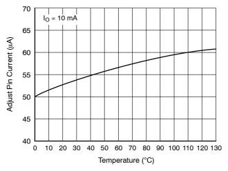
Figure 7. Adjust Pin Current vs. Temperature
