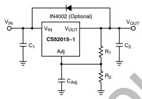
Figure 13. Protection Diode for Large Output Capacitors
