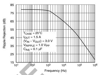
Figure 8. Ripple Rejection vs. Frequency
