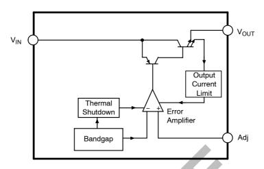
Figure 2. Block Diagram
