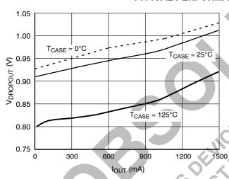
Figure 3. Dropout Voltage vs. Output Current
