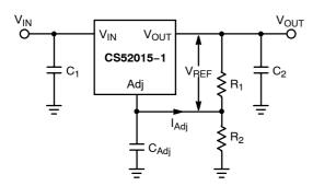
Figure 11. Resistor Divider Scheme
