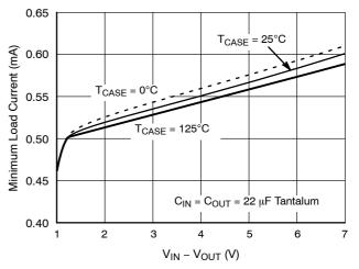
Figure 6. Minimum Load Current vs.  $V_{\text{IN}}$  –  $V_{\text{OUT}}$
