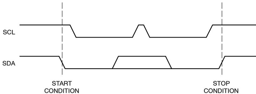
Figure 2. Start/Stop Timing
