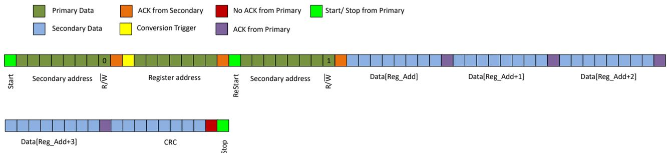
**Figure 7-10. Standard 3-Byte I<sup>2</sup>C Read With CRC Enabled, CRC\_EN = 1b**
