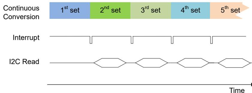
**Figure 8-10. Continuous Conversion With AC Line Power**
