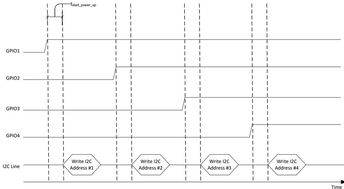
**Figure 8-14. Power-Up Timing and I<sup>2</sup>C Address Allocation for the Four Sensors**
