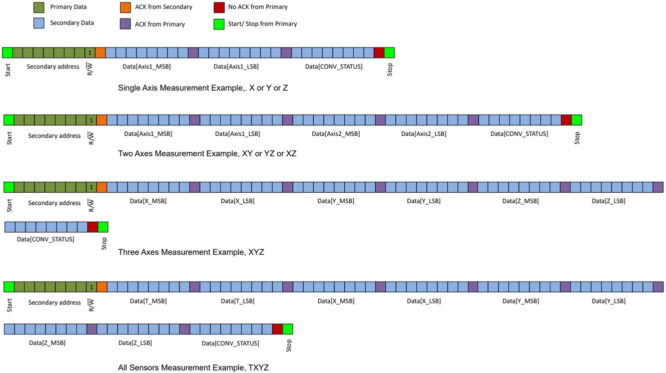
**Figure 7-11. 1-Byte I<sup>2</sup>C Read Command for 16-Bit Data With CRC Disabled, CRC\_EN = 0b**
