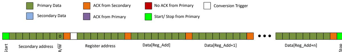
**Figure 7-7. Standard I<sup>2</sup>C Write**
