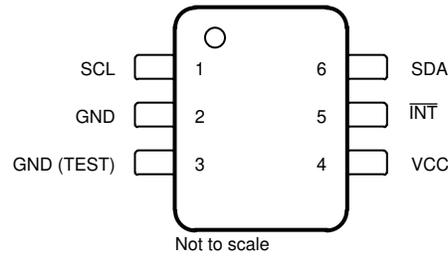
**Figure 5-1. DBV Package, 6-Pin SOT-23 (Top View)**
