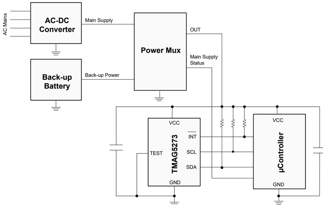
Figure 8-9. TMAG5273 Application Diagram for Tamper Detection
