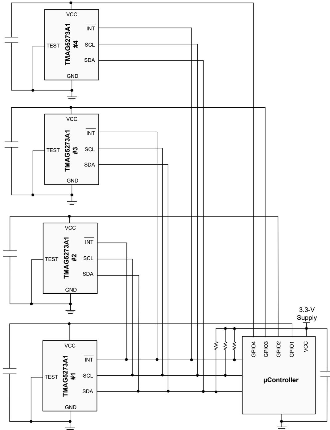
Figure 8-13. TMAG5273 Application Diagram for I<sup>2</sup>C Address Expansion
