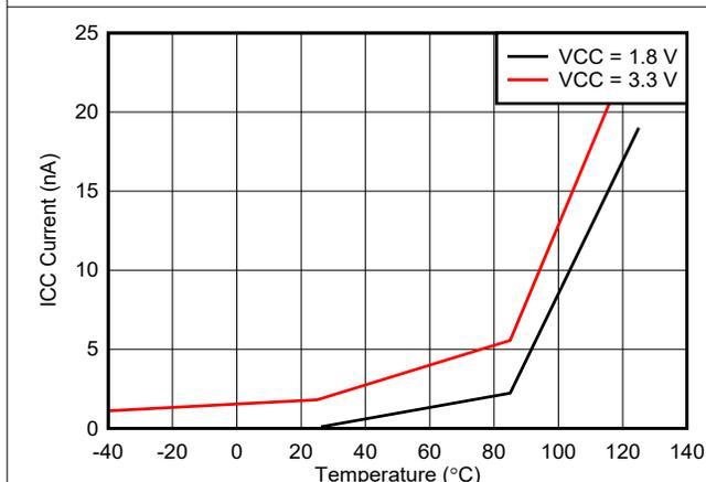
**Figure 6-3. Sleep Mode ICC vs. Temperature**
