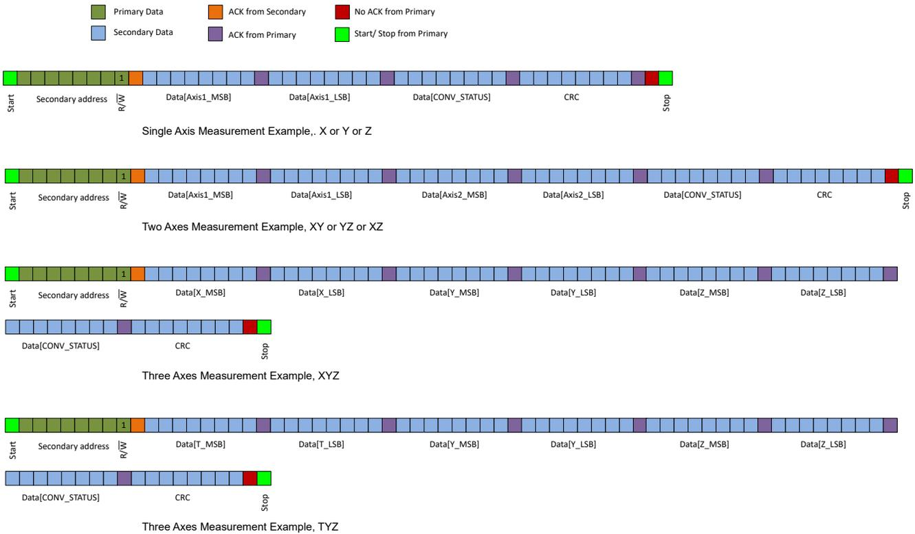
**Figure 7-12. 1-Byte I<sup>2</sup>C Read Command for 16-Bit Data With CRC Enabled, CRC\_EN = 1b**
