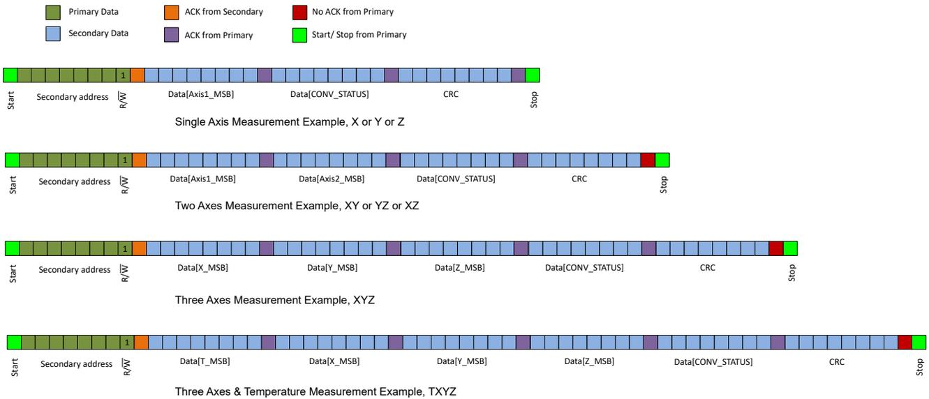
**Figure 7-14. 1-Byte I<sup>2</sup>C Read Command for 8-Bit Data With CRC Enabled, CRC\_EN = 1b**
