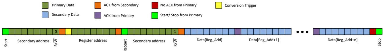
**Figure 7-9. Standard 3-Byte I<sup>2</sup>C Read With CRC Disabled, CRC\_EN = 0b**
