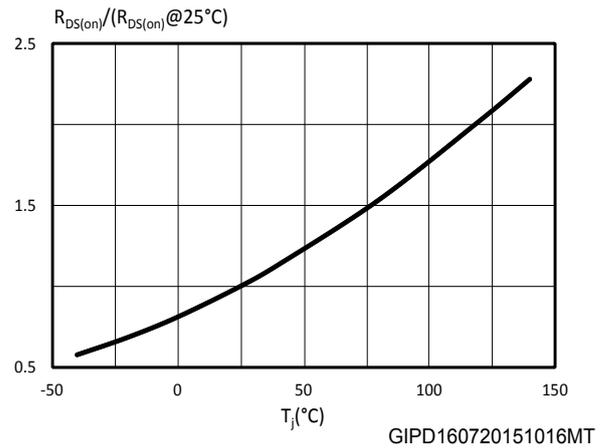
**Figure 19. Static drain source on resistance**
