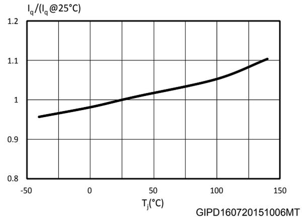
**Figure 9. Operating current  $I_{CC}$  vs  $T_J$**
