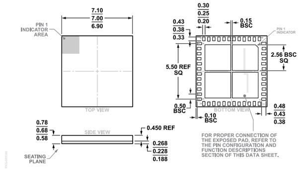
Figure 33. 48-Terminal Land Grid Array [LGA] (CC-48-1)
