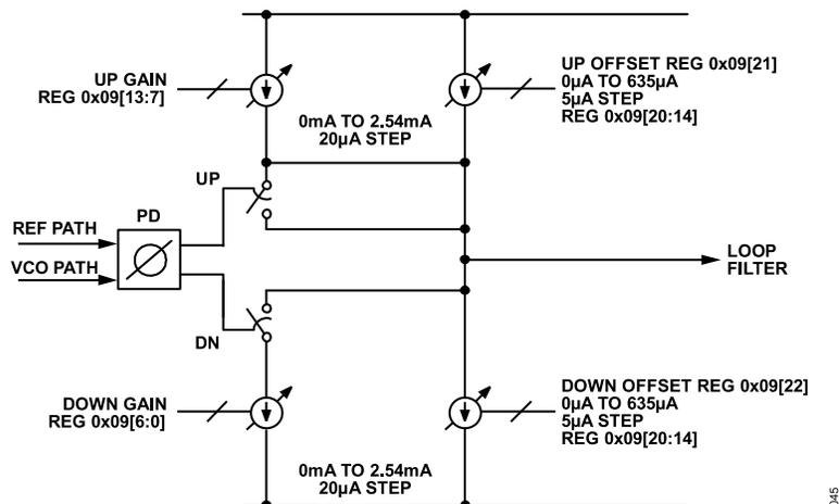
Figure 24. Charge Pump Gain and Offset Control
