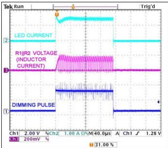
Figure 12. Dimming pulse of ~150µs.
