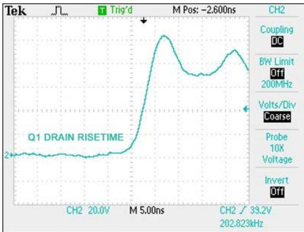
Figure 8. Drain voltage risetime.
