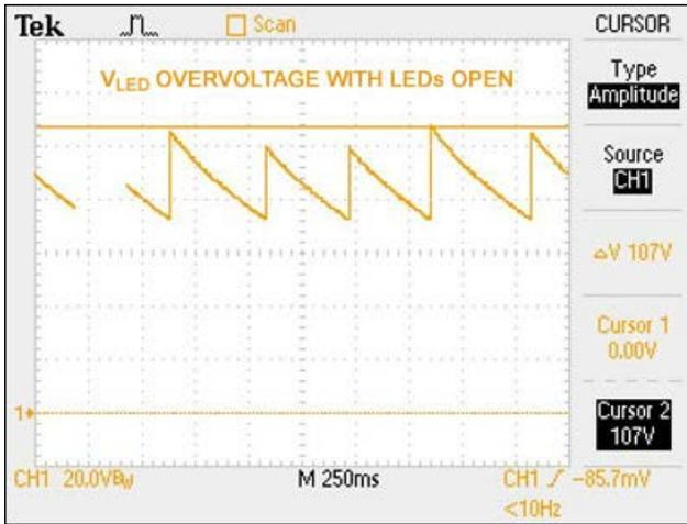
Figure 14. OVP with open LED string.
