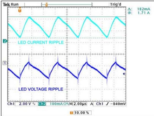
Figure 10. LED voltage (AC coupled) and current ripple.
