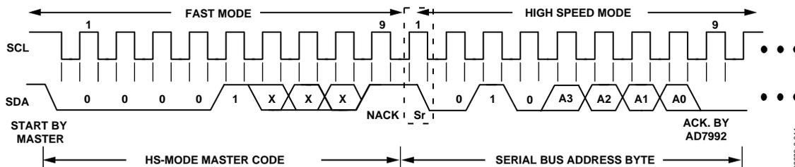
Figure 30. Placing the Part into High Speed Mode
