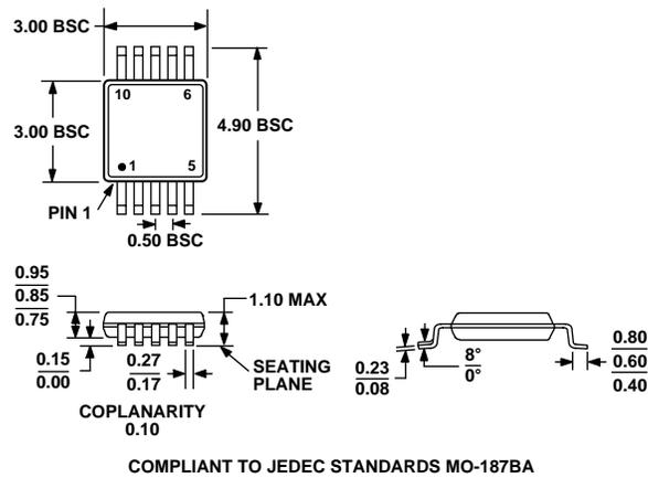
Figure 34. 10-Lead Mini Small Outline Package [MSOP]
