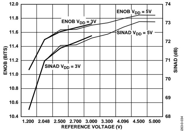
Figure 16. ENOB/SINAD vs. Reference Voltage, Mode 1, 121 kSPS
