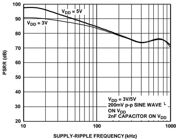
Figure 6. PSRR vs. Supply-Ripple Frequency, Single-Channel Mode Only
