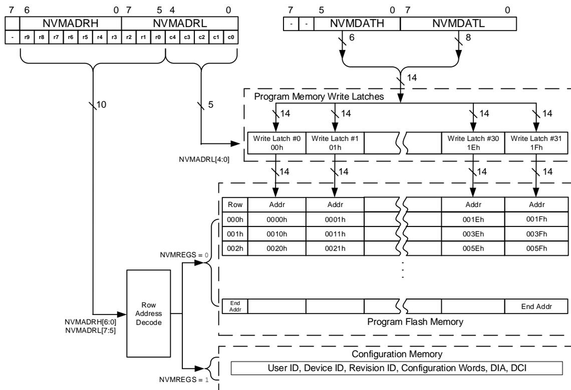
Figure 15-5. Program Flash Memory Write Sequence
