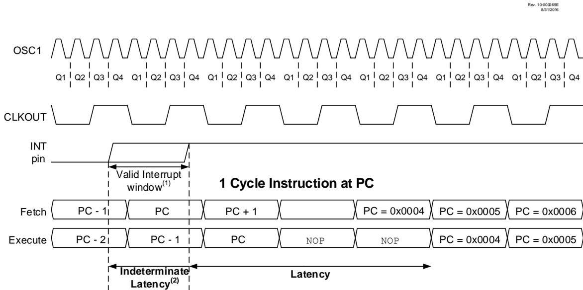
Figure 12-3. INT Pin Interrupt Timing
