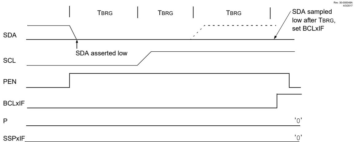
**Figure 25-41. Bus Collision During a Stop Condition (Case 2)**
