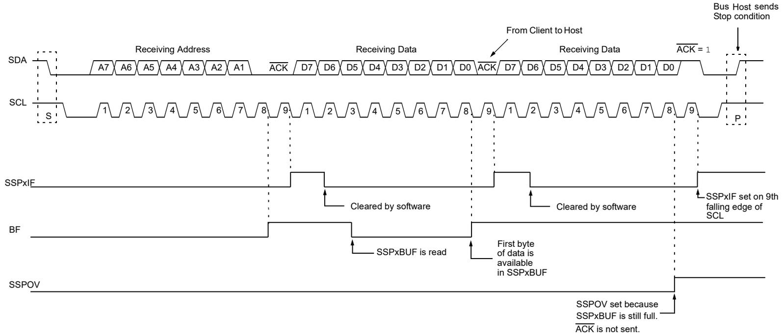
Figure 25-17. I<sup>2</sup>C Client, 7-Bit Address, Reception (SEN = 1, AHEN = 0, DHEN = 0)
