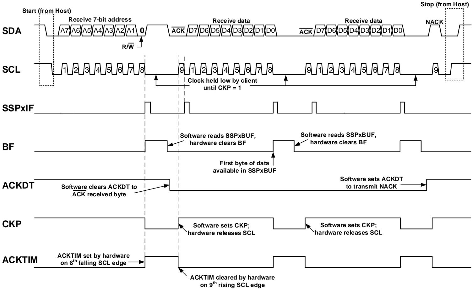
Figure 25-19. I<sup>2</sup>C Client, 7-Bit Address, Reception (SEN = 1, AHEN = 1, DHEN = 1)
