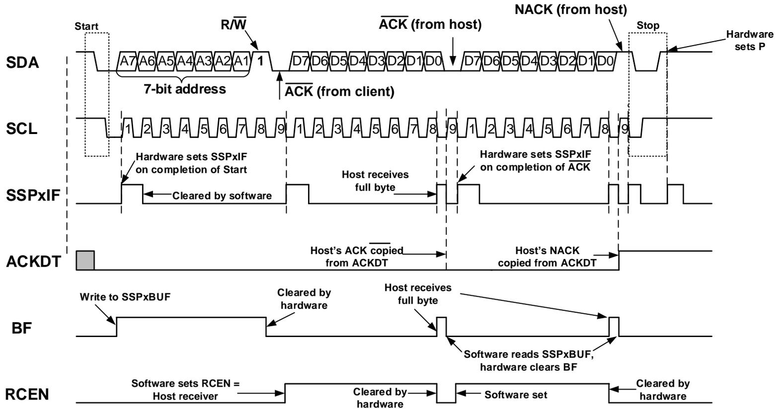
**Figure 25-33. I<sup>2</sup>C Host Mode Waveform (Reception, 10-Bit Address)**
