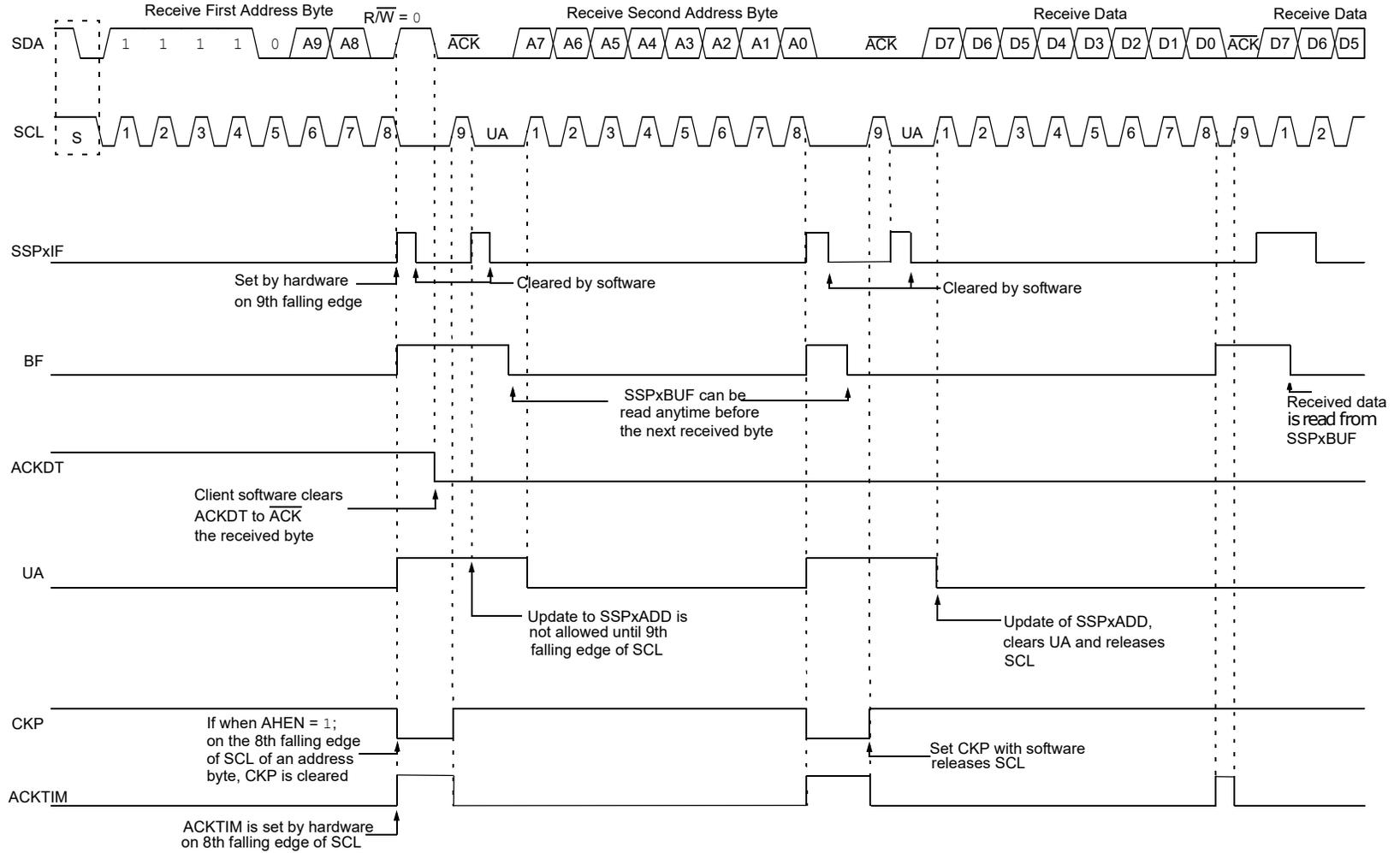
Figure 25-22. I<sup>2</sup>C Client, 10-Bit Address, Transmission (SEN = 0, AHEN = 0, DHEN = 0)
