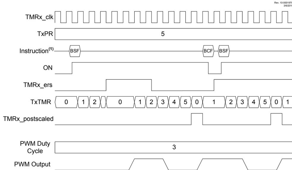
Note 1: BSF and BCF represent Bit-Set File and Bit-Clear File instructions executed by the CPU to set or clear the ON bit of TxCON. CPU execution is asynchronous to the timer clock input.
