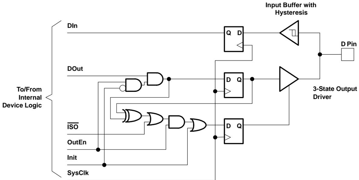
**Figure 15. Input/Output Differentiation Logic**
