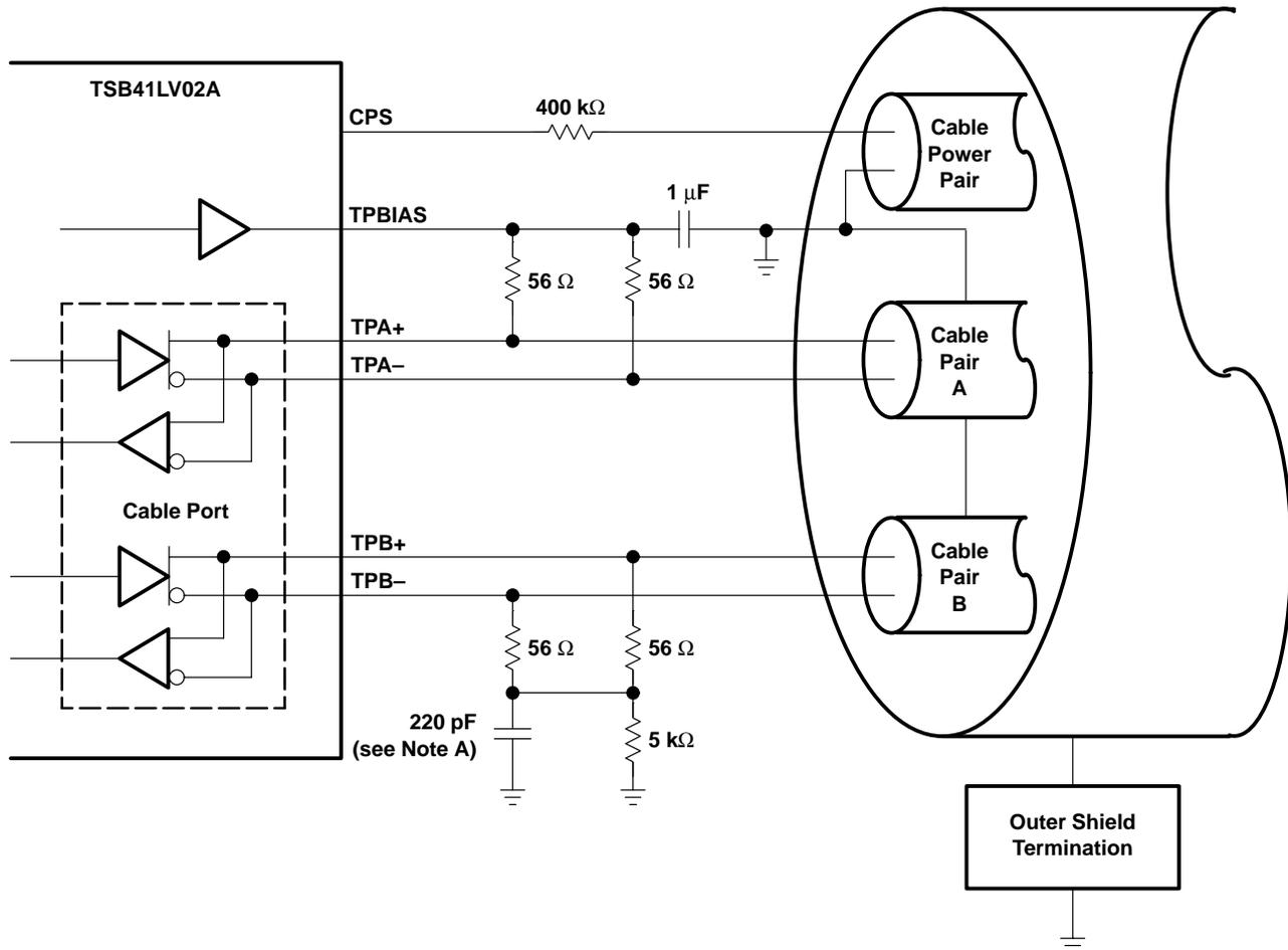
NOTE A: The IEEE Std 1394-1995 calls for a 250-pF capacitor, which is a nonstandard component value. A 220-pF capacitor is recommended.
