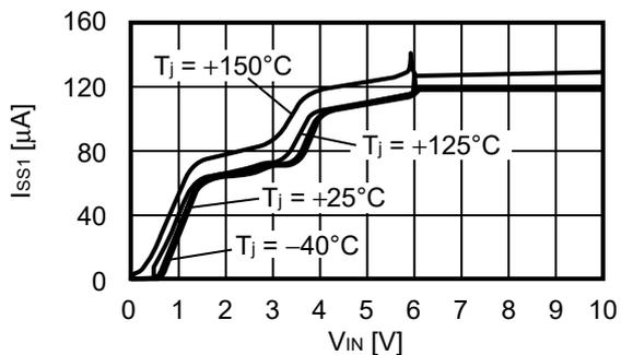
**8. Current consumption during operation vs. Junction temperature**
