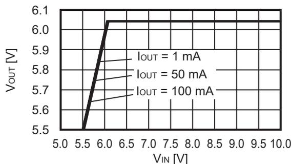
**3. Dropout voltage vs. Output current**
