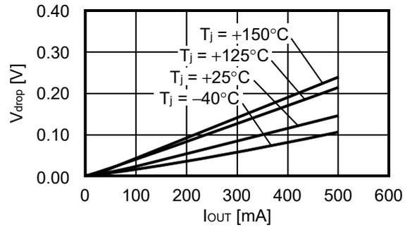
**4. Dropout voltage vs. Junction temperature**
