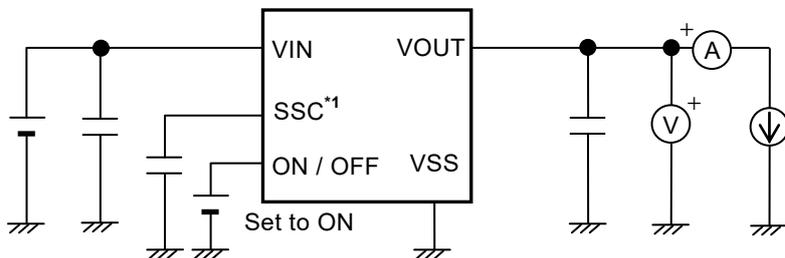
Figure 10 Test Circuit 1
