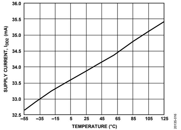
Figure 15. Supply Current ( $I_{DD2}$ ) vs. Temperature
