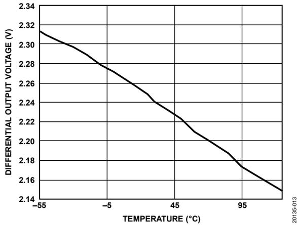
Figure 12. Differential Output Voltage vs. Temperature,  $R_L = 60\ \Omega$
