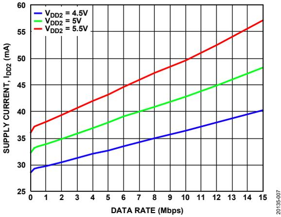
Figure 6. Supply Current ( $I_{DD2}$ ) vs. Data Rate
