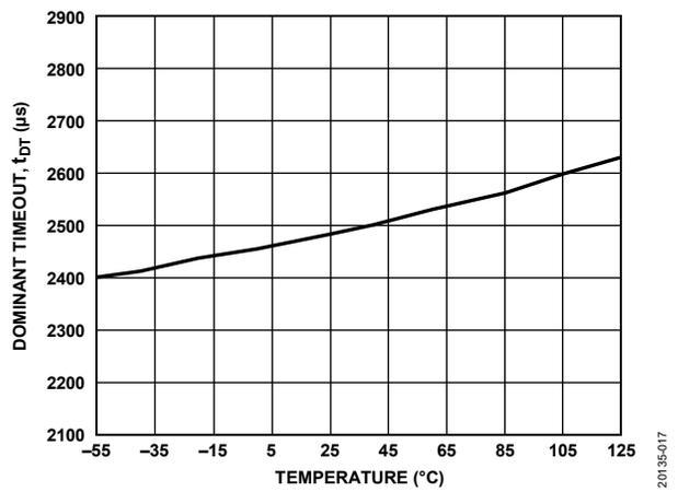
Figure 16. Dominant Timeout ( $t_{DT}$ ) vs. Temperature
