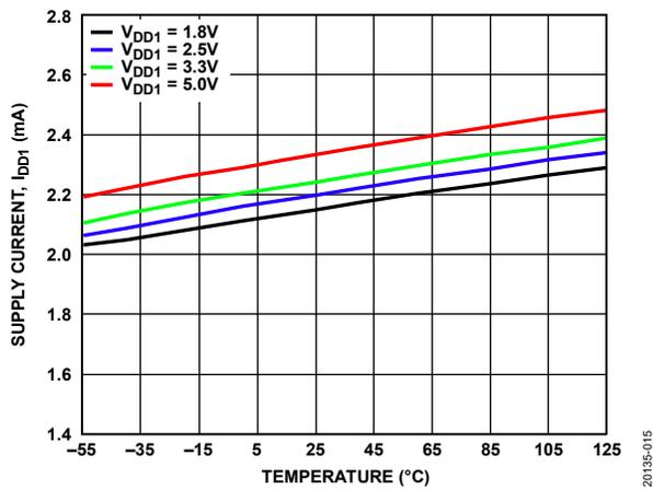
Figure 14. Supply Current ( $I_{DD1}$ ) vs. Temperature
