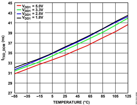
Figure 8.  $t_{TXD\_DOM}$  vs. Temperature
