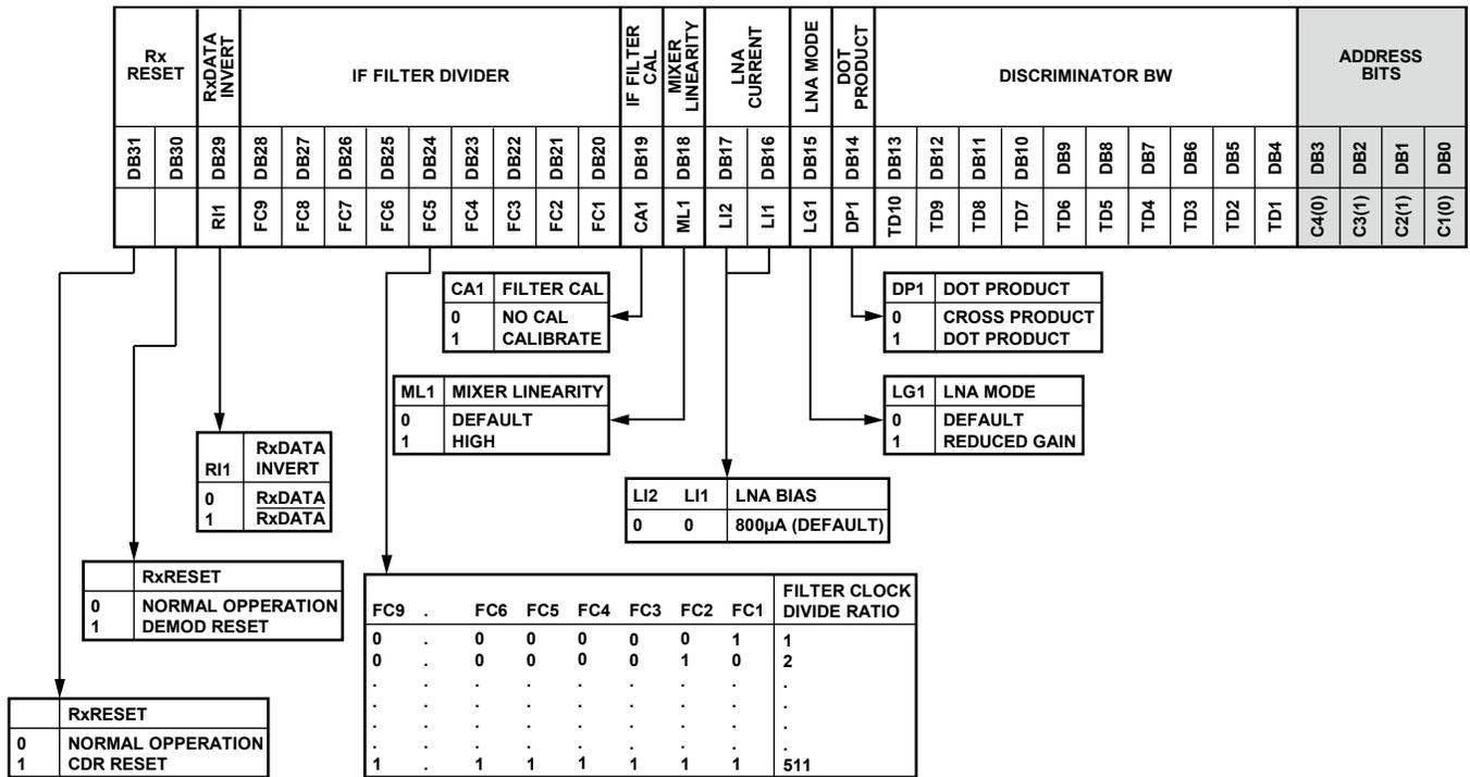
Figure 51. Register 6—Correlator/Demodulator Register
