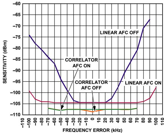
Figure 18. Sensitivity vs. Frequency Error with AFC On/Off
