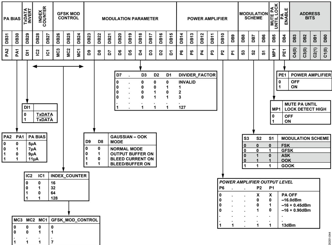
Figure 47. Register 2—Transmit Modulation Register (GFSK/GOOK Mode)
