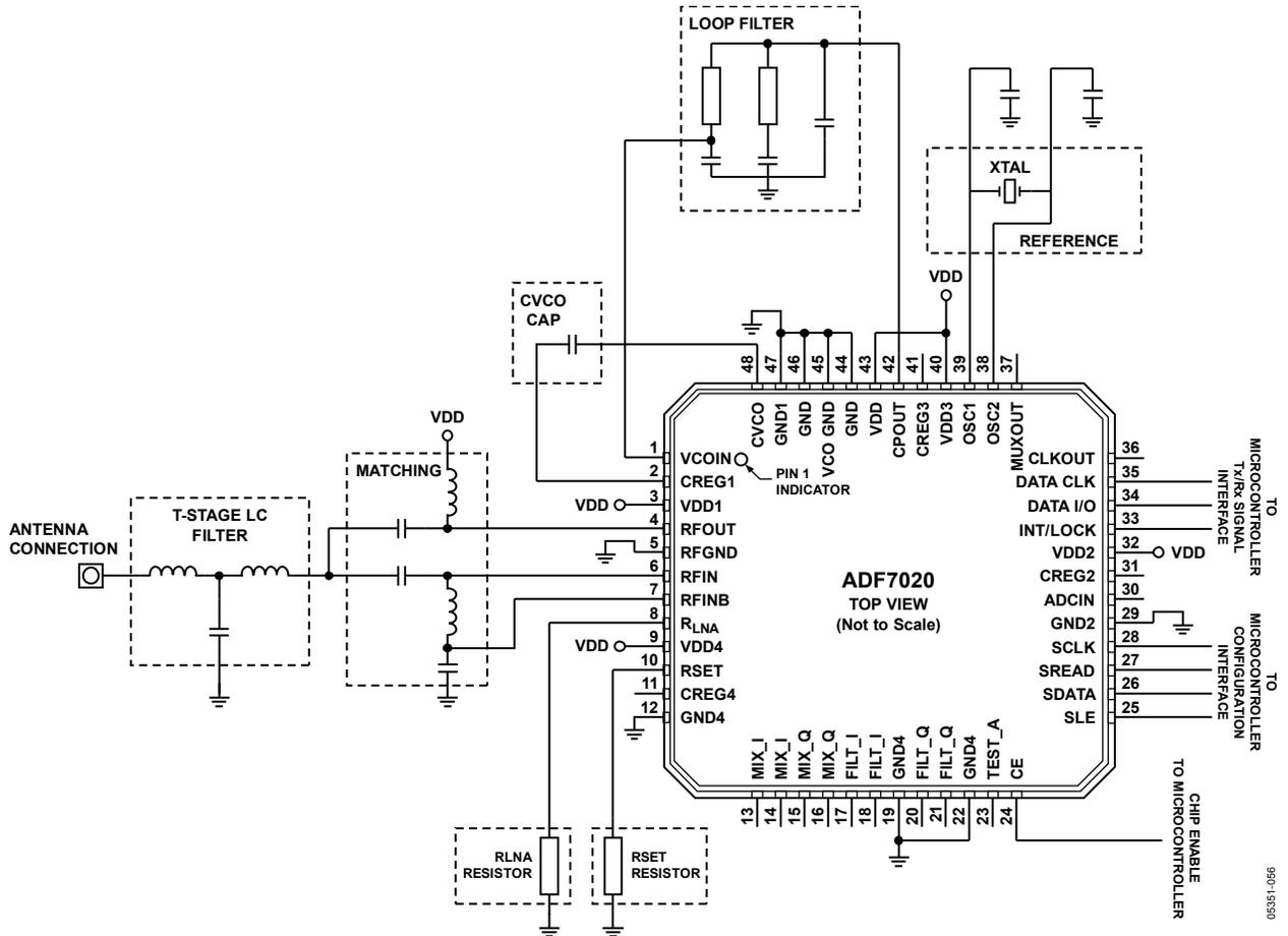
Figure 41. Application Circuit
