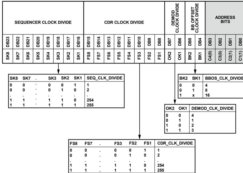
Figure 48. Register 3—Receiver Clock Register
