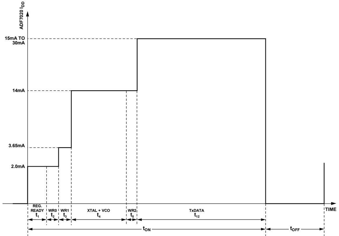
Figure 40. Tx Programming Sequence and Timing Diagram
