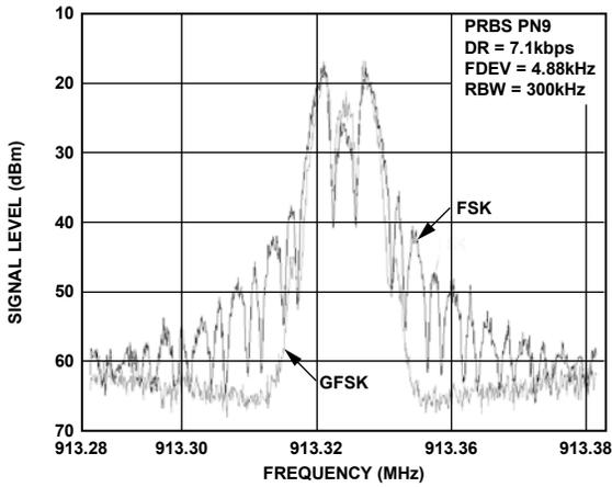
Figure 8. Output Spectrum in FSK and GFSK Modulation
