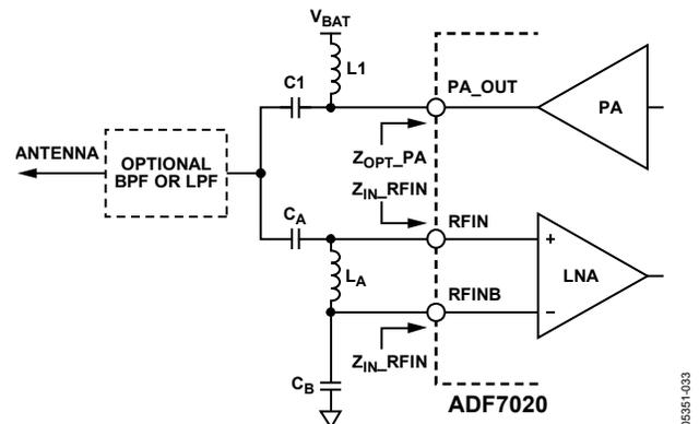
Figure 33. ADF7020 with Internal Rx/Tx Switch
