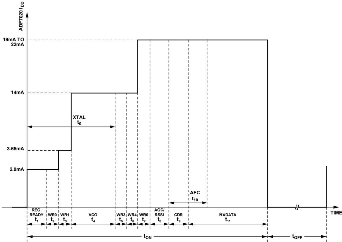
Figure 39. Rx Programming Sequence and Timing Diagram
