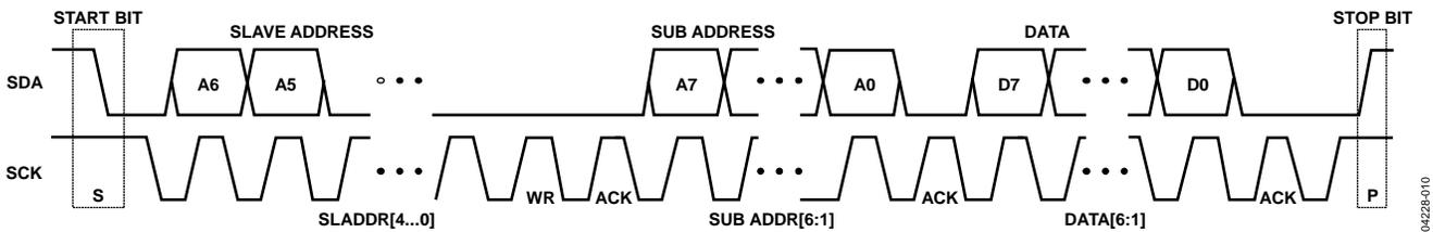
Figure 10. I<sup>2</sup>C Data Transfer Timing
