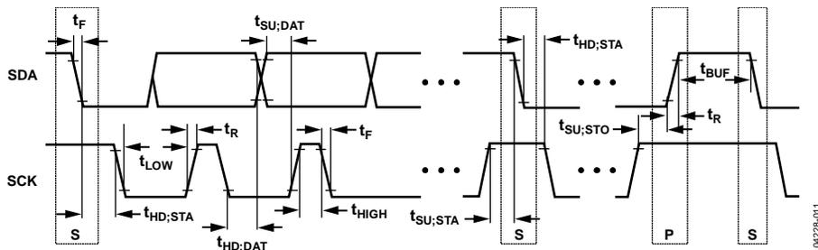
Figure 11. I<sup>2</sup>C Port Timing Diagram
