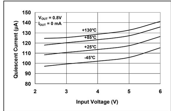
**FIGURE 2-10:** Quiescent Current vs. Input Voltage (0.8V Fixed).
