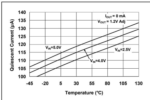
**FIGURE 2-3:** Quiescent Current vs. Junction Temperature (1.2V Adjustable).
