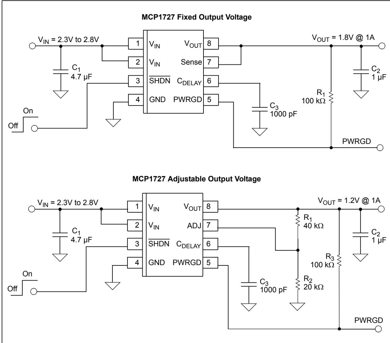
Functional Block Diagram - Adjustable Output
