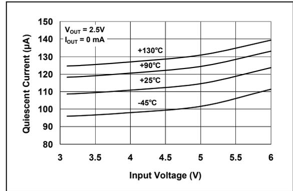
**FIGURE 2-11:** Quiescent Current vs. Input Voltage (2.5V Fixed).
