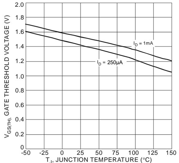
Figure 6. Gate Threshold Variation vs. Junction Temperature
