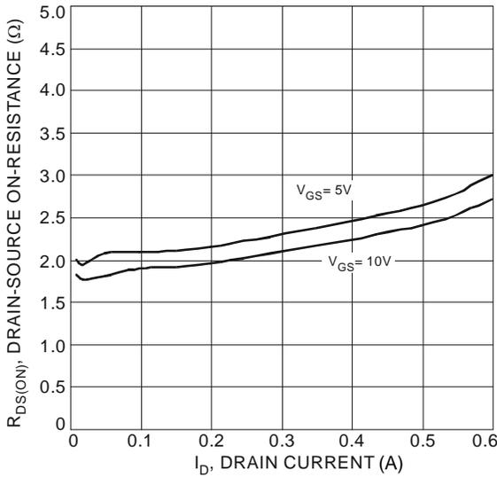
Figure 3. Typical On-Resistance vs. Drain Current and Temperature
