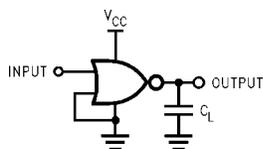
C<sub>L</sub> includes load and stray capacitance
