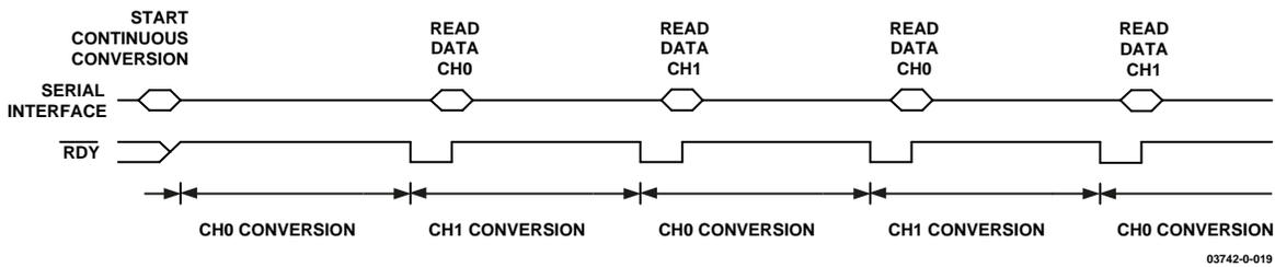
Figure 18. Continuous Conversion, CH0 and CH1, RDYFN = 0
