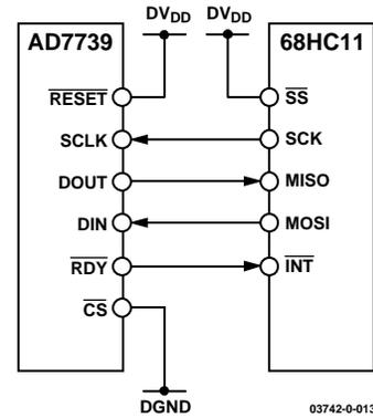
Figure 12. AD7739 to Host Device Interface, SPI
