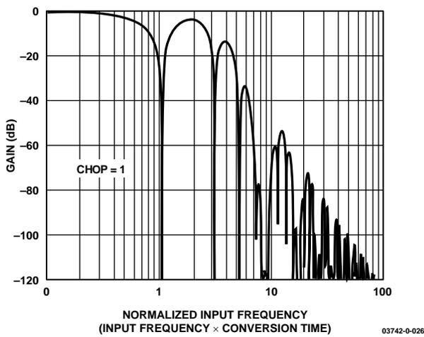
Figure 25. Typical ADC Frequency Response, Chopping Enabled
