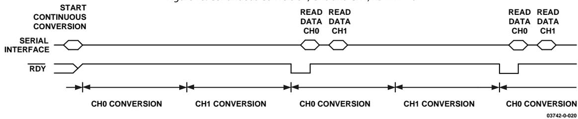
Figure 19. Continuous Conversion, CH0 and CH1, RDYFN = 1
