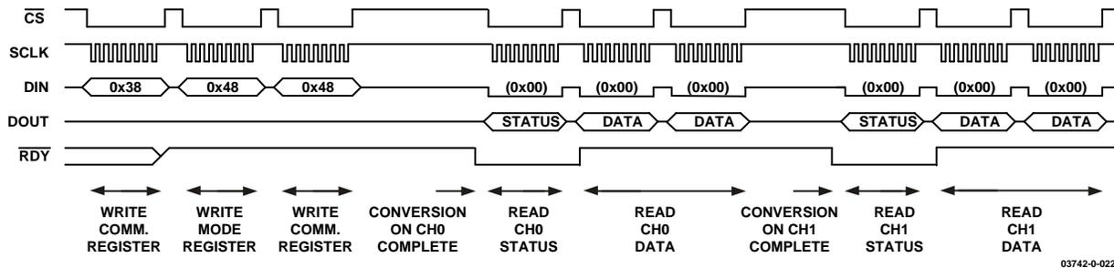
Figure 21. Continuous Conversion, CH0 and CH1, Continuous Read
