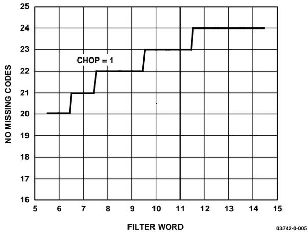
Figure 6. No Missing Codes Performance, Chopping Enabled
