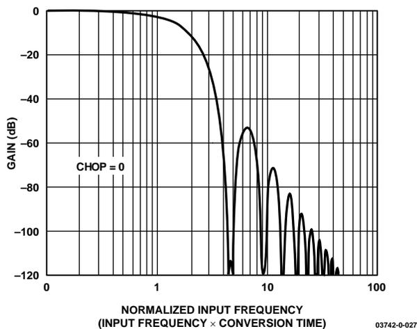
Figure 26. Typical ADC Frequency Response, Chopping Disabled
