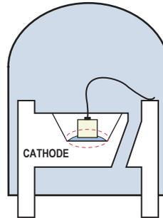
Note: Electrical connection between bottom surface of LED die and the lead frame is achieved through conductive paste.
