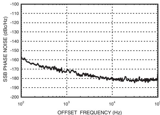
**Phase Noise at Pout = Psat @ 9 GHz**
