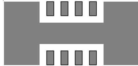
(e) Copper Area = 70mm<sup>2</sup>,  $\theta_{JA} = 49^{\circ}\text{C/W}$
