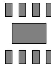
(b) Copper Area = 10mm<sup>2</sup>,  $\theta_{JA} = 64^\circ\text{C/W}$
