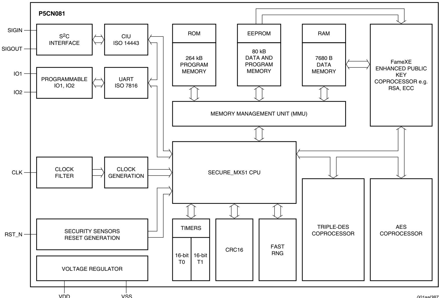
Fig 3. Functional diagram P5CN081
