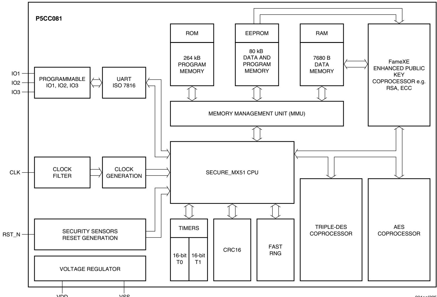
Fig 1. Functional diagram P5CC081
