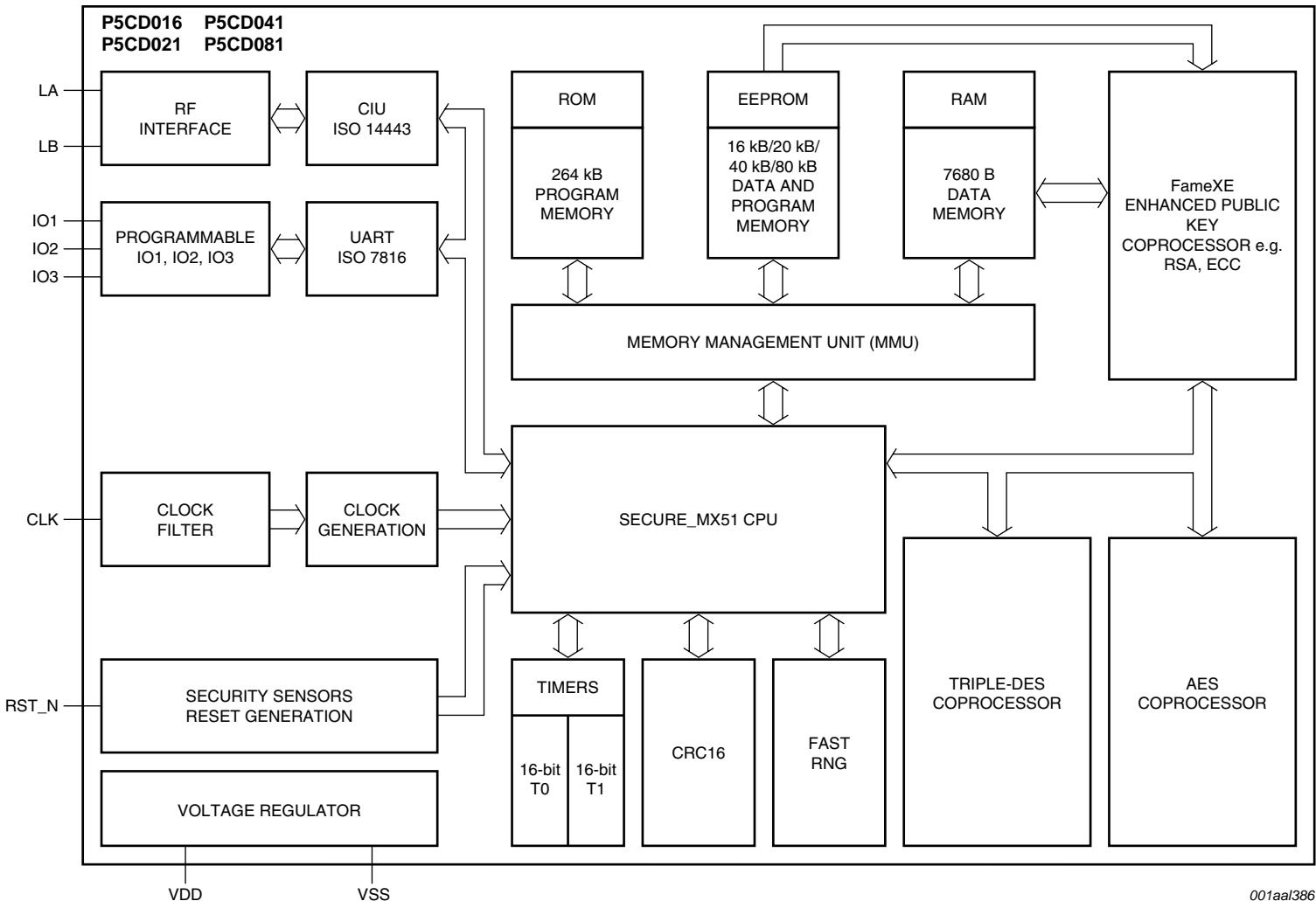
Fig 2. Functional diagram P5CD016/P5CD021/P5CD041/P5CD081
