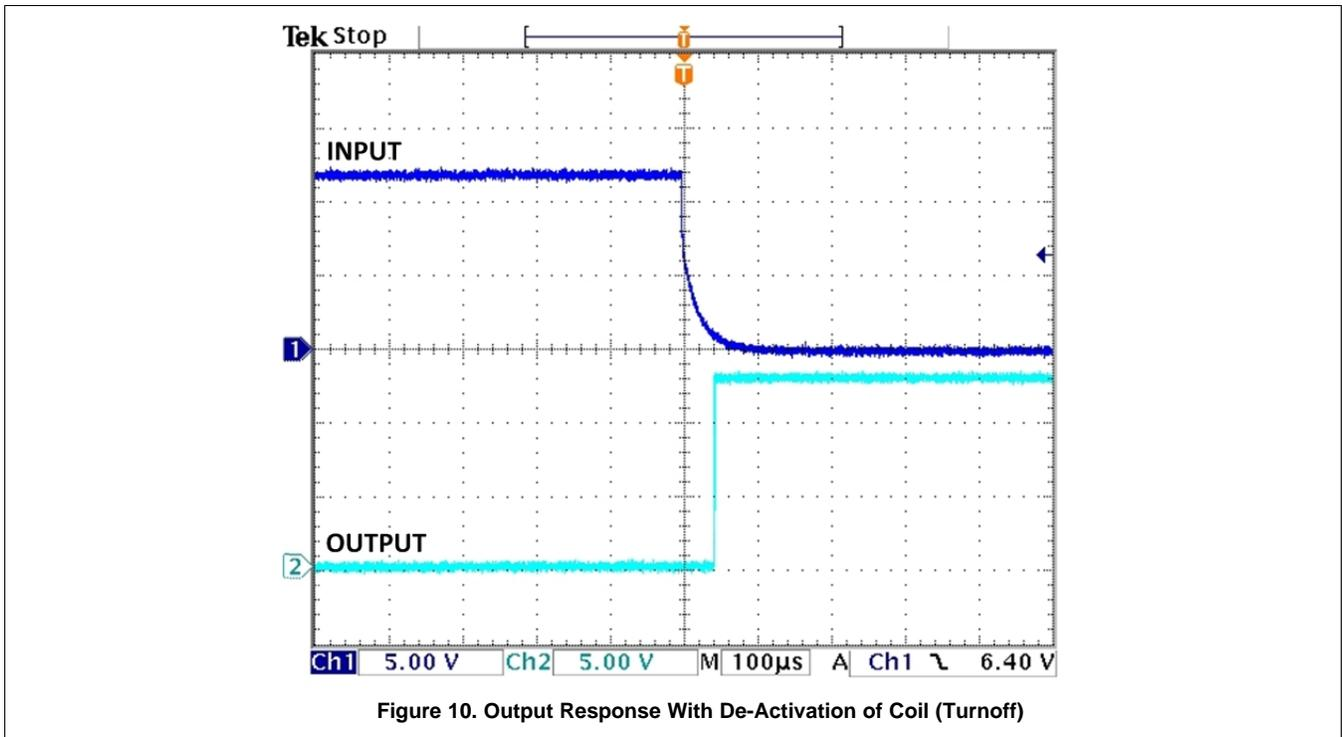
Figure 10. Output Response With De-Activation of Coil (Turnoff)
