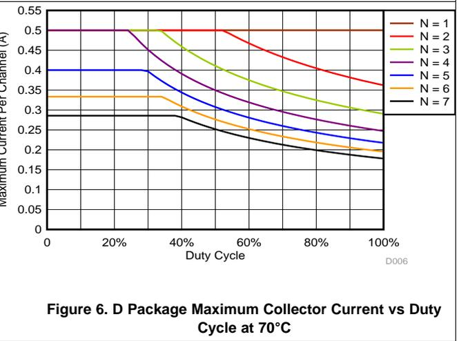
Figure 6. D Package Maximum Collector Current vs Duty Cycle at 70°C
