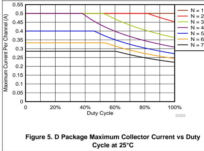
Figure 5. D Package Maximum Collector Current vs Duty Cycle at 25°C
