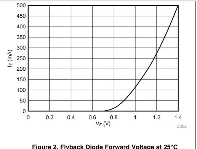
Figure 2. Flyback Diode Forward Voltage at 25°C
