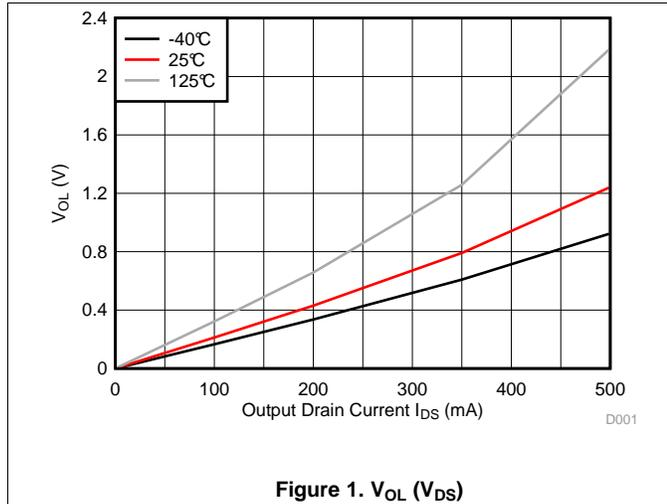
Figure 1.  $V_{OL}$  ( $V_{DS}$ )
