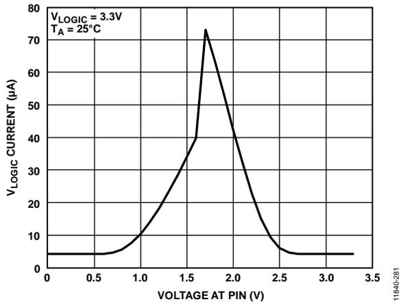
Figure 69.  $V_{Logic}$  Current vs. Logic Input Voltage
