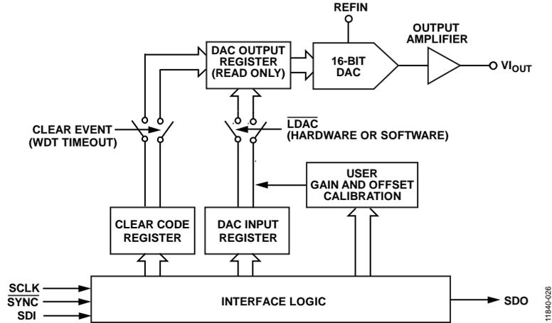
Figure 82. Simplified Serial Interface of Input Loading Circuitry
