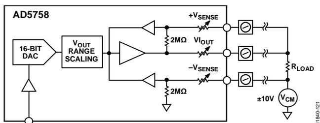
Figure 78. Voltage Output
