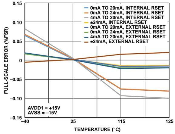
Figure 40. Full-Scale Error vs. Temperature
