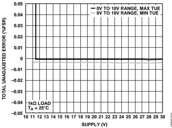
Figure 20. Total Unadjusted Error vs.  $AV_{DD1}/AV_{SS}$  Supply
