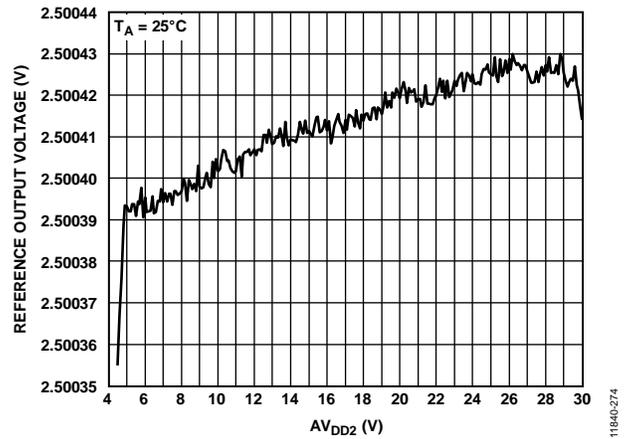
Figure 67. Reference Output Voltage vs. AV<sub>DD2</sub> Supply
