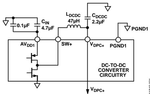
Figure 77. DC-to-DC Circuit
