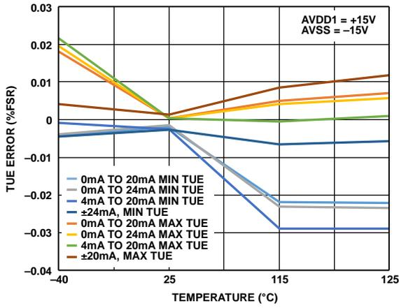
Figure 38. Total Unadjusted Error vs. Temperature, External RSET
