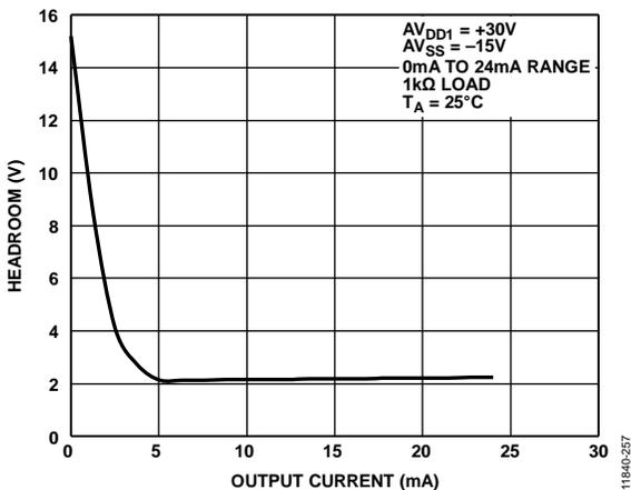
Figure 51. DC-to-DC Converter Headroom vs. Output Current
