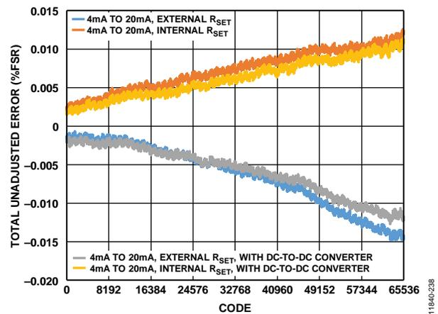
Figure 33. Total Unadjusted Error vs. DAC Code
