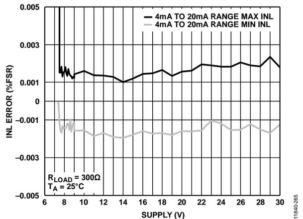
Figure 47. INL Error vs.  $AV_{DD1}/|AV_{SS}|$  Supply, Internal  $R_{SET}$
