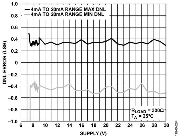
Figure 45. DNL Error vs.  $AV_{DD1}/|AV_{SS}|$  Supply, Internal  $R_{SET}$
