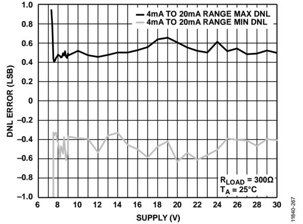
Figure 46. DNL Error vs.  $AV_{DD1}/|AV_{SS}|$  Supply, External  $R_{SET}$
