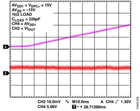
Figure 28.  $V_{OUT}$  vs. Time on Power Up
