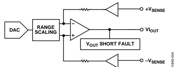
Figure 75. Voltage Output
