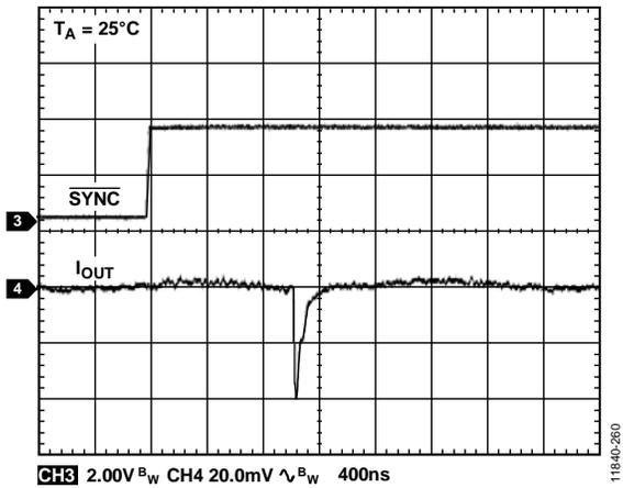
Figure 50. Output Current vs. Time on Output Enable
