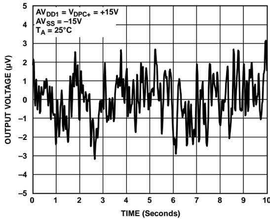
Figure 64. Peak-to-Peak Noise (0.1 Hz to 10 Hz Bandwidth)
