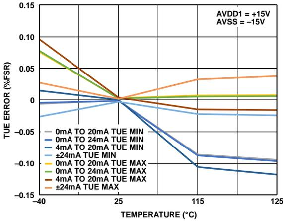
Figure 37. Total Unadjusted Error vs. Temperature, Internal RSET
