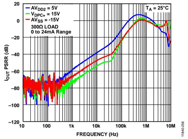
Figure 56.  $I_{OUT}$  PSRR vs. Frequency
