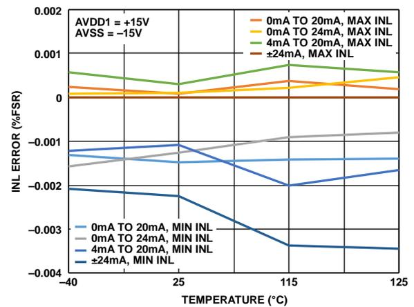
Figure 35. INL Error vs. Temperature, External  $R_{SET}$
