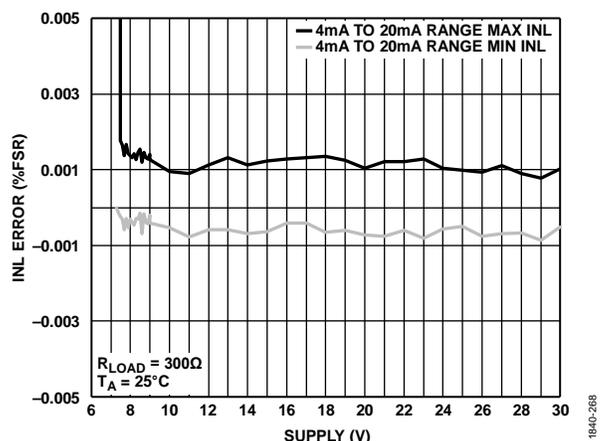
Figure 48. INL Error vs.  $AV_{DD1}/|AV_{SS}|$  Supply, External  $R_{SET}$
