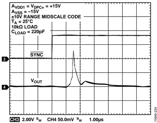
Figure 27.  $V_{OUT}$  vs. Time on Output Enable
