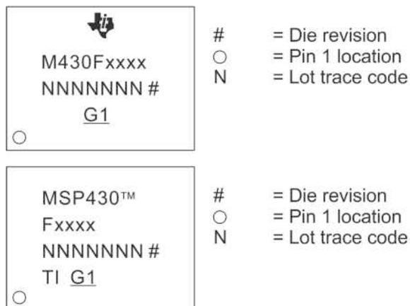
NOTE: Package marking with "TM" applies only to devices released after 2011.
