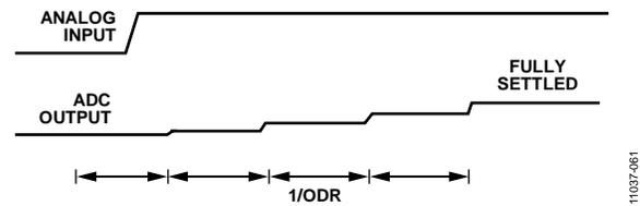
Figure 54. Step Input Without Single Cycle Settling
