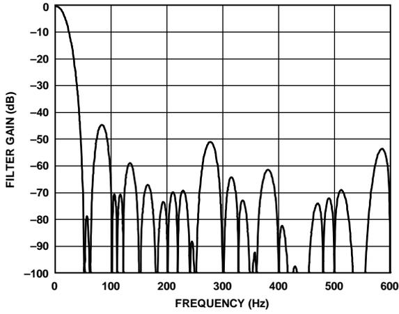
Figure 62. 16.667 SPS ODR, 60 ms Settling Time
