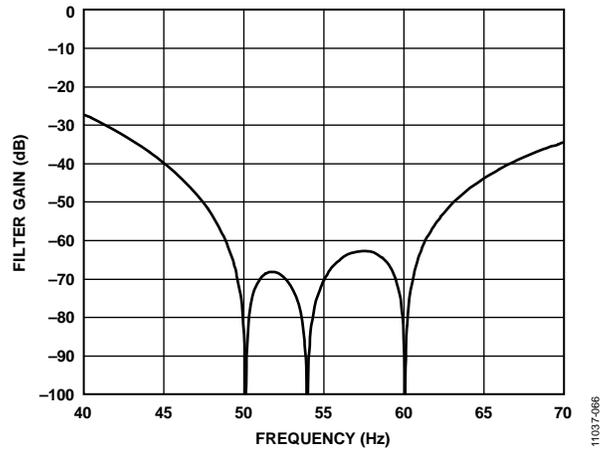
Figure 60. 25 SPS ODR, 40 ms Settling Time
