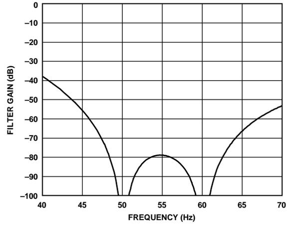
Figure 63. 16.667 SPS ODR, 60 ms Settling Time
