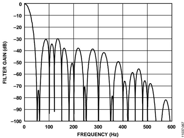
Figure 58. 20 SPS ODR, 50 ms Settling Time
