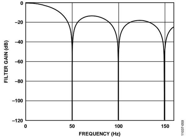
Figure 52. Sinc5 + Sinc1 Filter Response at 50 SPS ODR
