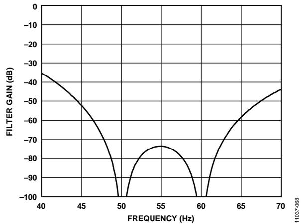
Figure 61. 20 SPS ODR, 50 ms Settling Time
