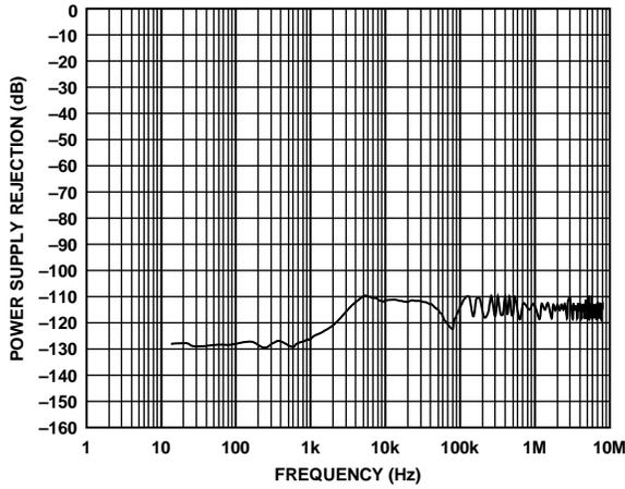
Figure 23. Power Supply Rejection Ratio vs. Frequency
