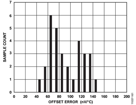
Figure 32. Offset Error Drift Distribution Histogram (Internal Short)
