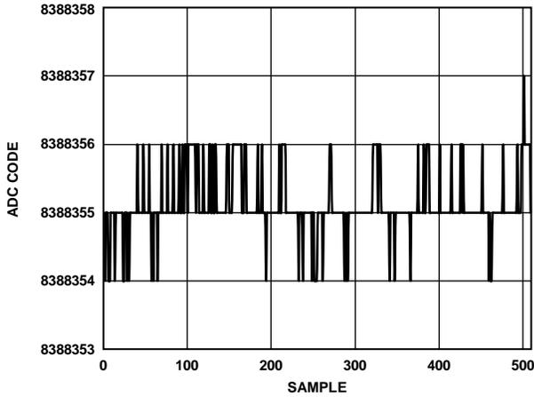
Figure 5. Noise ( $V_{REF} = 5 V$ , Output Data Rate = 5 SPS)
