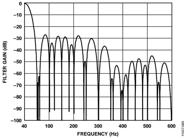
Figure 57. 25 SPS ODR, 40 ms Settling Time
