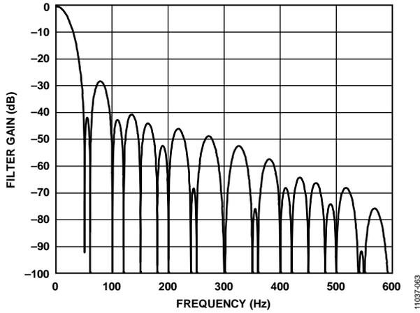
Figure 56. 27.27 SPS ODR, 36.67 ms Settling Time
