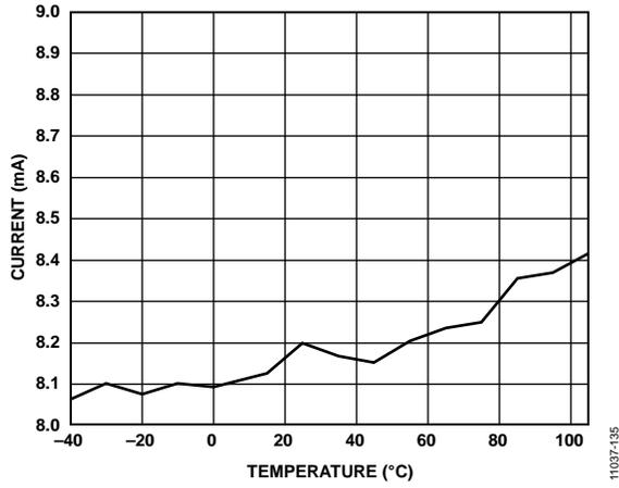
Figure 35. Current Consumption vs Temperature (Continuous Conversion Mode)
