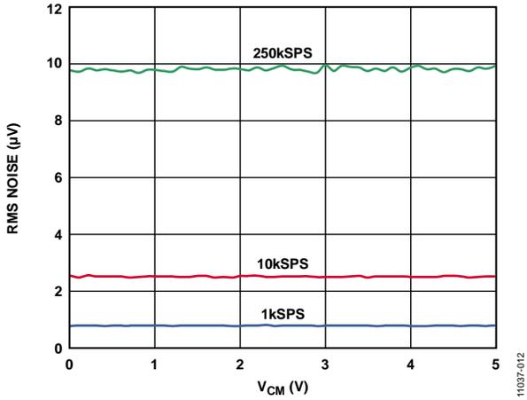
Figure 11. Noise vs. Common-Mode Input Voltage ( $V_{REF} = 2.5 V$ )
