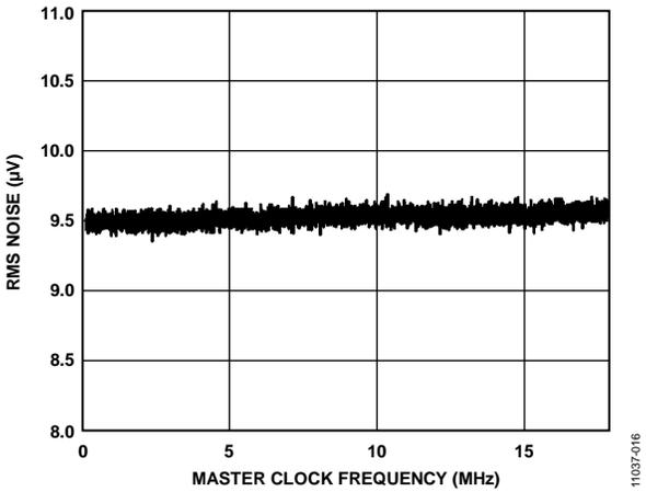
Figure 12. Noise vs. Master Clock ( $V_{REF} = 2.5 V$ )
