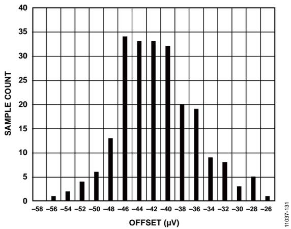
Figure 31. Offset Error Distribution Histogram (Internal Short)
