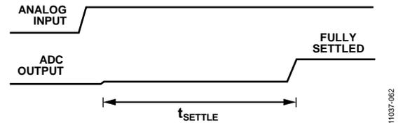
Figure 55. Step Input with Single Cycle Settling
