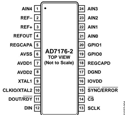
Figure 4. Pin Configuration
