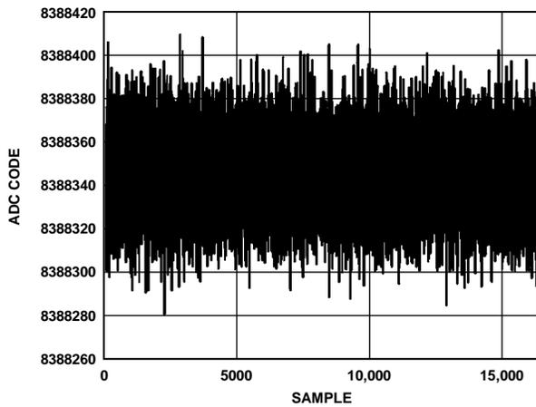
Figure 7. Noise ( $V_{REF} = 5 V$ , Output Data Rate = 250 kSPS)
