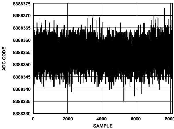
Figure 6. Noise ( $V_{REF} = 5 V$ , Output Data Rate = 10 kSPS)
