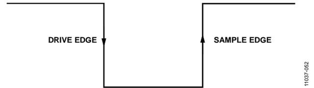
Figure 38. SPI Mode 3 SCLK Edges
