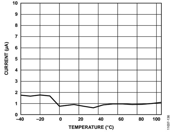
Figure 36. Current Consumption vs Temperature (Power Down Mode)
