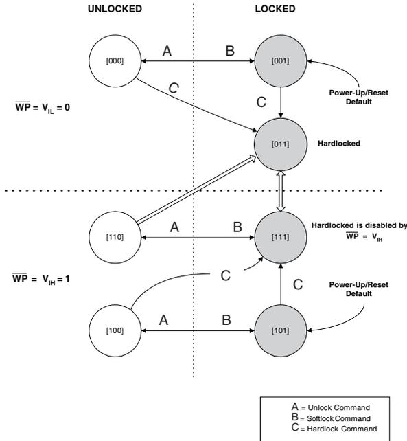
Note: 1. The notation [X, Y, Z] denotes the locking state of a sector. The current locking state of a sector is defined by the state of  $\overline{WP}$  and the two bits of the sector-lock status D[1:0].
