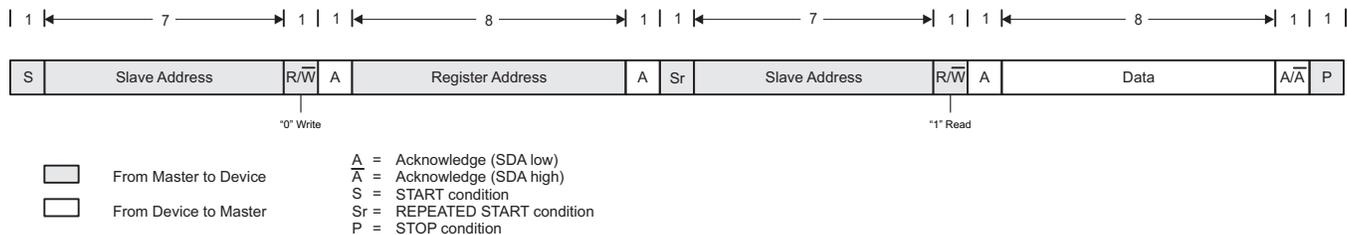
Figure 46. Read Data Transfer Format in F/S-Mode
