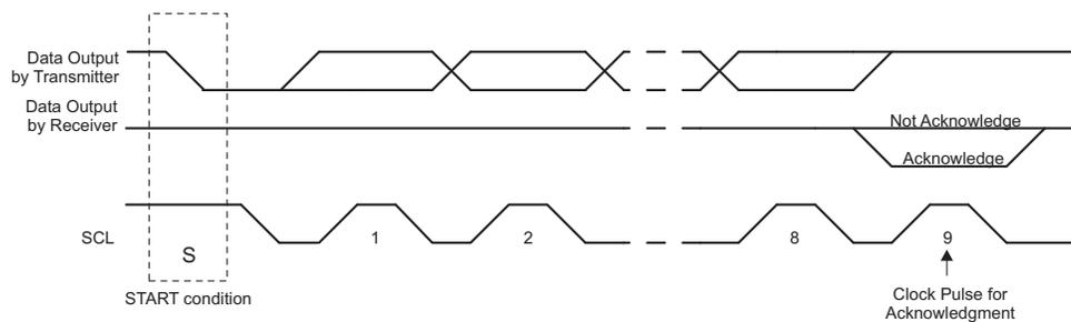
Figure 43. Acknowledge on the I<sup>2</sup>C Bus
