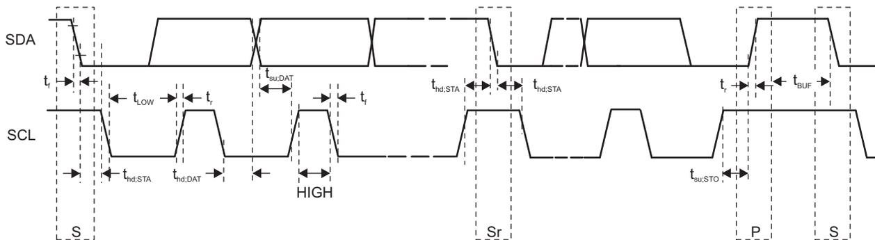
Figure 1. Serial Interface Timing for F/S Mode
