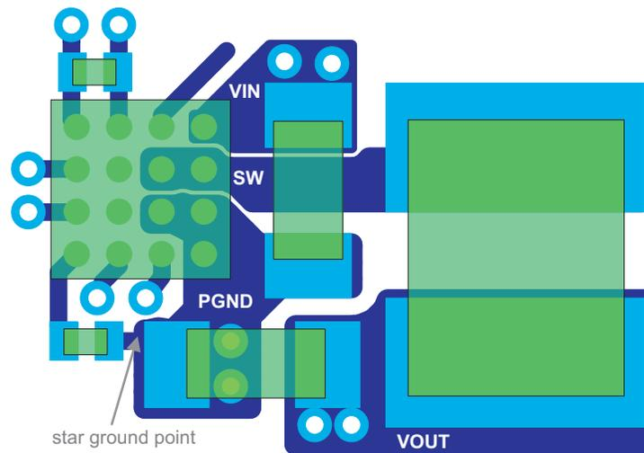
**Figure 52. Layout Suggestion (top view) with 3225 Inductor. Overall Solution Size: 27.5mm<sup>2</sup>**
