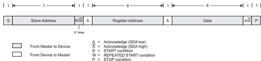
Figure 45. Write Data Transfer Format in F/S-Mode
