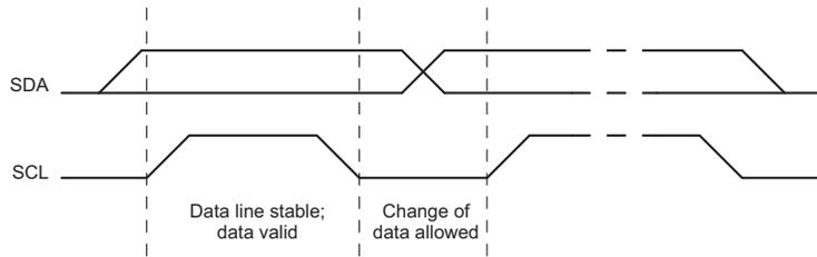
Figure 42. Bit Transfer on the Serial Interface
