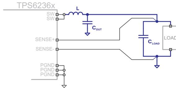
Figure 50. L, C<sub>OUT</sub> and C<sub>LOAD</sub> Forming the Output Filter
