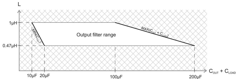
Figure 51. Recommended L, C<sub>OUT</sub> and C<sub>LOAD</sub> Combinations
