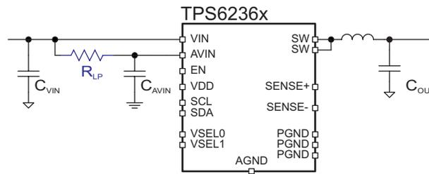
Figure 49. Optional Low Pass Filter at AVIN
