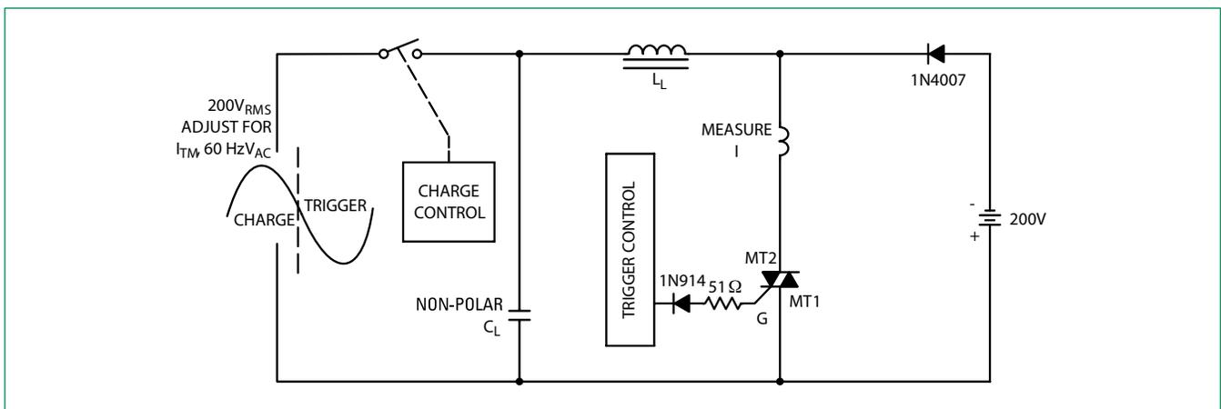
Note: Component values are for verification of rated ( $di/dt$ ). See AN1048 for additional information
