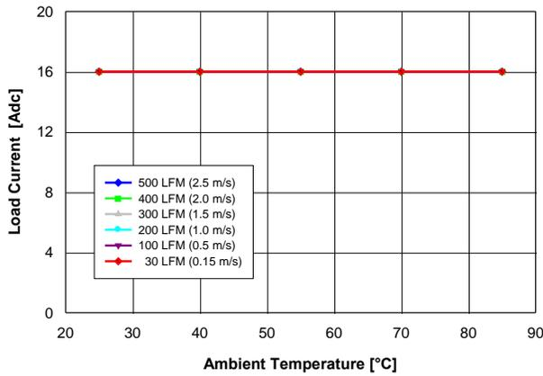
Fig. 1.8V.1: Available load current vs. ambient temperature and airflow rates for  $V_{out} = 1.8\text{ V}$  converter mounted vertically with  $V_{in} = 5\text{ V}$ , and maximum MOSFET temperature  $\leq 120\text{ }^\circ\text{C}$ .
