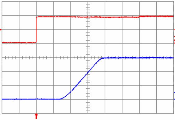
Fig. 1.5V.5: Turn-on transient for  $V_{out} = 1.5\text{ V}$  with the application of Enable signal at full rated load current (resistive) and  $47\text{ }\mu\text{F}$  external capacitance at  $V_{in} = 5\text{ V}$ . Top trace: Enable signal (2 V/div.); Bottom trace: output voltage (500 mV/div.); Time scale: 2 ms/div.
