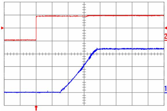
Fig. 0.7525V.5: Turn-on transient for  $V_{out} = 0.7525\text{ V}$  with the application of Enable signal at full rated load current (resistive) and  $47\text{ }\mu\text{F}$  external capacitance at  $V_{in} = 5\text{ V}$ . Top trace: Enable signal (2 V/div.); Bottom trace: output voltage (200 mV/div.); Time scale: 2 ms/div.
