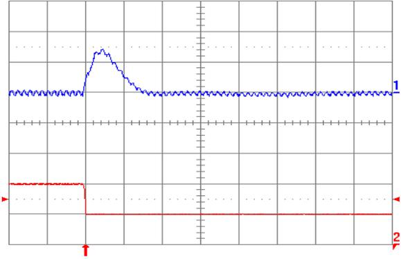
Fig. 2.0V.8: Output voltage response for  $V_{out} = 2.0\text{ V}$  to negative load current step change from 10 A to 5 A with slew rate of  $-5\text{ A}/\mu\text{s}$  at  $V_{in} = 5\text{ V}$ . Top trace: output voltage (100 mV/div.); Bottom trace: load current (5 A/div.).  $C_o = 47\text{ }\mu\text{F}$  ceramic +  $1\text{ }\mu\text{F}$  ceramic. Time scale:  $20\text{ }\mu\text{s}/\text{div}$ .
