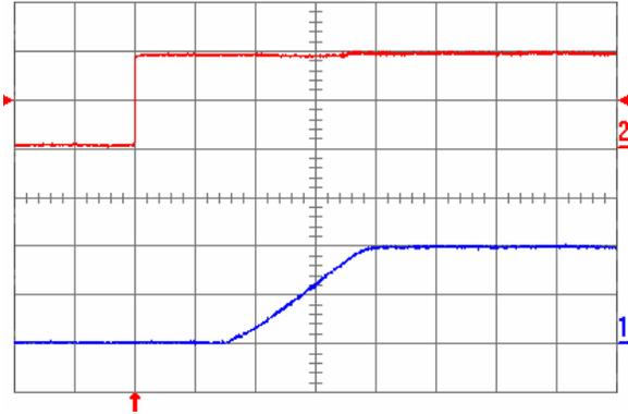
Fig. 1.0V.5: Turn-on transient for  $V_{out} = 1.0\text{ V}$  with the application of Enable signal at full rated load current (resistive) and  $47\ \mu\text{F}$  external capacitance at  $V_{in} = 5\text{ V}$ . Top trace: Enable signal (2 V/div.); Bottom trace: output voltage (500 mV/div.); Time scale: 2 ms/div.
