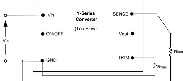
Fig. E: Configuration for programming output voltage.
