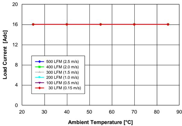
Fig. 2.5V.1: Available load current vs. ambient temperature and airflow rates for  $V_{out} = 2.5\text{ V}$  converter mounted vertically with  $V_{in} = 5\text{ V}$ , and maximum MOSFET temperature  $\leq 120\text{ }^\circ\text{C}$ .
