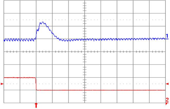
Fig. 1.2V.8: Output voltage response for  $V_{out} = 1.2\text{ V}$  to negative load current step change from 10 A to 5 A with slew rate of  $-5\text{ A}/\mu\text{s}$  at  $V_{in} = 5\text{ V}$ . Top trace: output voltage (100 mV/div.); Bottom trace: load current (5 A/div.).  $C_o = 47\text{ }\mu\text{F}$  ceramic +  $1\text{ }\mu\text{F}$  ceramic. Time scale:  $20\text{ }\mu\text{s}/\text{div}$ .
