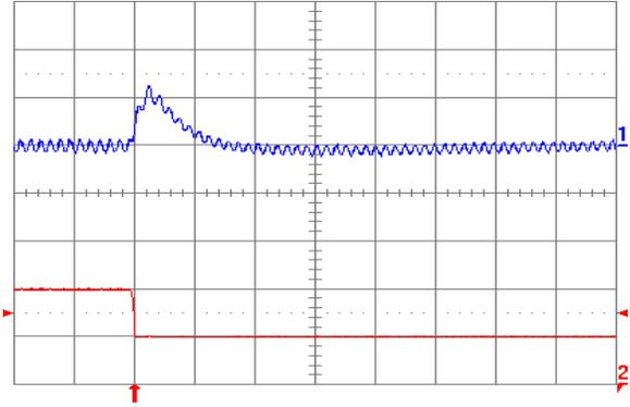
Fig. 3.3V.8: Output voltage response for  $V_{out} = 3.3\text{ V}$  to negative load current step change from 10 A to 5 A with slew rate of  $-5\text{ A}/\mu\text{s}$  at  $V_{in} = 5\text{ V}$ . Top trace: output voltage (100 mV/div.); Bottom trace: load current (5 A/div.).  $C_o = 47\text{ }\mu\text{F}$  ceramic +  $1\text{ }\mu\text{F}$  ceramic. Time scale:  $20\text{ }\mu\text{s}/\text{div}$ .
