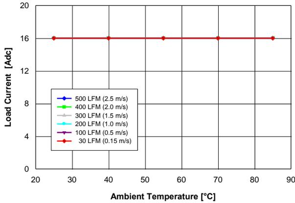
Fig. 3.3V.1: Available load current vs. ambient temperature and airflow rates for  $V_{out} = 3.3\text{ V}$  converter mounted vertically with  $V_{in} = 5\text{ V}$ , and maximum MOSFET temperature  $\leq 120^\circ\text{C}$ .
