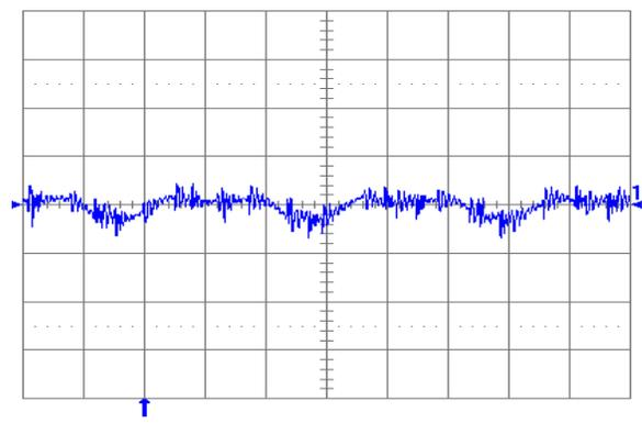
Fig. 1.2V.6: Output voltage ripple (20 mV/div.) at full rated load current into a resistive load with external capacitance  $47\text{ }\mu\text{F}$  ceramic +  $1\text{ }\mu\text{F}$  ceramic, and  $V_{in} = 5\text{ V}$  for  $V_{out} = 1.2\text{ V}$ . Time scale: 2 μs/div.
