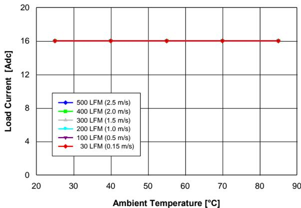
Fig. 1.5V.1: Available load current vs. ambient temperature and airflow rates for  $V_{out} = 1.5\text{ V}$  converter mounted vertically with  $V_{in} = 5\text{ V}$ , and maximum MOSFET temperature  $\leq 120\text{ }^\circ\text{C}$ .
