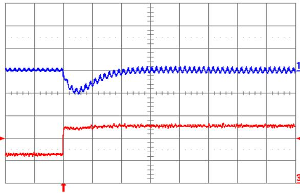
Fig. 1.0V.7: Output voltage response  $V_{out} = 1.0\text{ V}$  to positive load current step change from 5 A to 10 A with slew rate of  $5\text{ A}/\mu\text{s}$  at  $V_{in} = 5\text{ V}$ . Top trace: output voltage (100 mV/div.); Bottom trace: load current (5 A/div.).  $C_o = 47\ \mu\text{F}$  ceramic +  $1\ \mu\text{F}$  ceramic. Time scale: 20  $\mu\text{s}$ /div.
