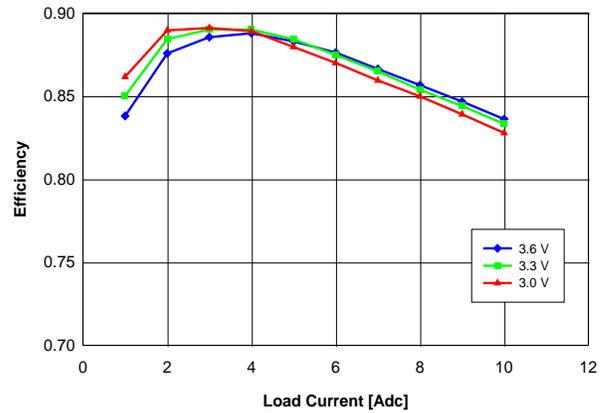
Fig. 0.7525V.4: Efficiency vs. load current and input voltage for  $V_{out} = 0.7525\text{ V}$  converter mounted vertically with air flowing at a rate of 200 LFM (1 m/s) and  $T_a = 25\text{ }^\circ\text{C}$ .
