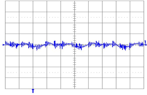
Fig. 1.0V.6: Output voltage ripple (20 mV/div.) at full rated load current into a resistive load with external capacitance  $47\ \mu\text{F}$  ceramic +  $1\ \mu\text{F}$  ceramic, and  $V_{in} = 5\text{ V}$  for  $V_{out} = 1.0\text{ V}$ . Time scale: 2  $\mu\text{s}$ /div.
