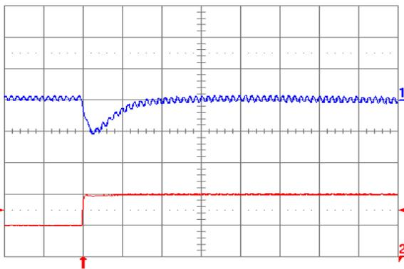
Fig. 2.5V.7: Output voltage response for  $V_{out} = 2.5\text{ V}$  to positive load current step change from 5 A to 10 A with slew rate of  $5\text{ A}/\mu\text{s}$  at  $V_{in} = 5\text{ V}$ . Top trace: output voltage (100 mV/div.); Bottom trace: load current (5 A/div.).  $C_o = 47\text{ }\mu\text{F}$  ceramic +  $1\text{ }\mu\text{F}$  ceramic. Time scale: 20  $\mu\text{s}$ /div.
