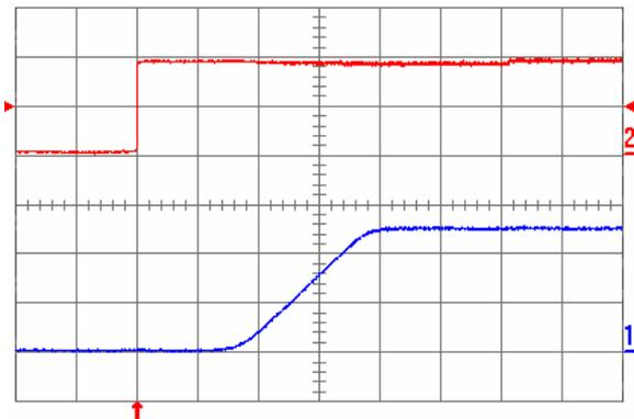
Fig. 2.5V.5: Turn-on transient for  $V_{out} = 2.5\text{ V}$  with the application of Enable signal at full rated load current (resistive) and  $47\text{ }\mu\text{F}$  external capacitance at  $V_{in} = 5\text{ V}$ . Top trace: Enable signal (2 V/div.); Bottom trace: output voltage (1 V/div.); Time scale: 2 ms/div.
