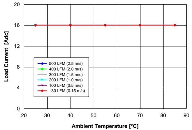
Fig. 2.5V.2: Available load current vs. ambient temperature and airflow rates for  $V_{out} = 2.5\text{ V}$  converter mounted horizontally with  $V_{in} = 5\text{ V}$ , and maximum MOSFET temperature  $\leq 120\text{ }^\circ\text{C}$ .
