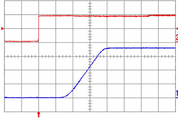
Fig. 1.8V.5: Turn-on transient for  $V_{out} = 1.8\text{ V}$  with the application of Enable signal at full rated load current (resistive) and  $47\text{ }\mu\text{F}$  external capacitance at  $V_{in} = 5\text{ V}$ . Top trace: Enable signal (2 V/div.); Bottom trace: output voltage (500 mV/div.); Time scale: 2 ms/div.
