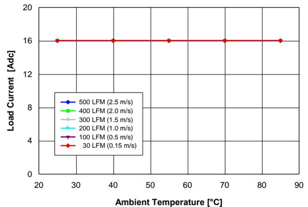
Fig. 1.5V.2: Available load current vs. ambient temperature and airflow rates for  $V_{out} = 1.5\text{ V}$  converter mounted horizontally with  $V_{in} = 5\text{ V}$ , and maximum MOSFET temperature  $\leq 120\text{ }^\circ\text{C}$ .
