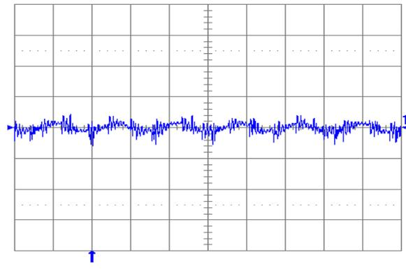
Fig. 1.5V.6: Output voltage ripple (20 mV/div.) at full rated load current into a resistive load with external capacitance  $47\text{ }\mu\text{F}$  ceramic +  $1\text{ }\mu\text{F}$  ceramic, and  $V_{in} = 5\text{ V}$  for  $V_{out} = 1.5\text{ V}$ . Time scale: 2  $\mu\text{s}$ /div.
