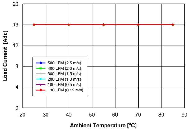
Fig. 1.0V.1: Available load current vs. ambient temperature and airflow rates for  $V_{out} = 1.0\text{ V}$  converter mounted vertically with  $V_{in} = 5\text{ V}$ , and maximum MOSFET temperature  $\leq 120\text{ }^\circ\text{C}$ .
