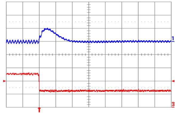
Fig. 1.0V.8: Output voltage response for  $V_{out} = 1.0\text{ V}$  to negative load current step change from 10 A to 5 A with slew rate of  $-5\text{ A}/\mu\text{s}$  at  $V_{in} = 5\text{ V}$ . Top trace: output voltage (100 mV/div.); Bottom trace: load current (5 A/div.).  $C_o = 47\ \mu\text{F}$  ceramic +  $1\ \mu\text{F}$  ceramic. Time scale: 20  $\mu\text{s}$ /div.
