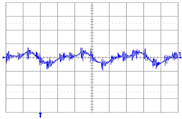
Fig. 2.5V.6: Output voltage ripple (20 mV/div.) at full rated load current into a resistive load with external capacitance  $47\text{ }\mu\text{F}$  ceramic +  $1\text{ }\mu\text{F}$  ceramic, and  $V_{in} = 5\text{ V}$  for  $V_{out} = 2.5\text{ V}$ . Time scale: 2  $\mu\text{s}$ /div.
