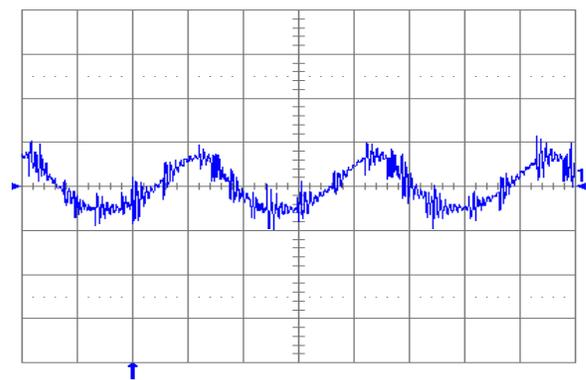
Fig. 3.3V.6: Output voltage ripple (20 mV/div.) at full rated load current into a resistive load with external capacitance  $47\ \mu\text{F}$  ceramic +  $1\ \mu\text{F}$  ceramic, and  $V_{in} = 5\text{ V}$  for  $V_{out} = 3.3\text{ V}$ . Time scale:  $2\ \mu\text{s}/\text{div}$ .
