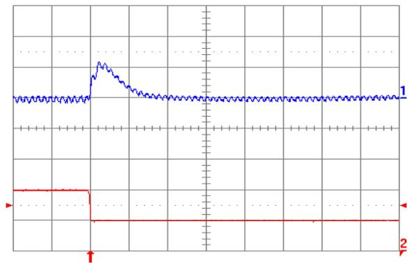
Fig. 2.5V.8: Output voltage response for  $V_{out} = 2.5\text{ V}$  to negative load current step change from 10 A to 5 A with slew rate of  $-5\text{ A}/\mu\text{s}$  at  $V_{in} = 5\text{ V}$ . Top trace: output voltage (100 mV/div.); Bottom trace: load current (5 A/div.).  $C_o = 47\text{ }\mu\text{F}$  ceramic +  $1\text{ }\mu\text{F}$  ceramic. Time scale: 20  $\mu\text{s}$ /div.
