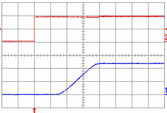
Fig. 1.2V.5: Turn-on transient for  $V_{out} = 1.2\text{ V}$  with the application of Enable signal at full rated load current (resistive) and  $47\text{ }\mu\text{F}$  external capacitance at  $V_{in} = 5\text{ V}$ . Top trace: Enable signal (2 V/div.); Bottom trace: output voltage (500 mV/div.); Time scale: 2 ms/div.
