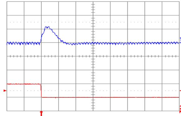
Fig. 1.5V.8: Output voltage response for  $V_{out} = 1.5\text{ V}$  to negative load current step change from 10 A to 5 A with slew rate of  $-5\text{ A}/\mu\text{s}$  at  $V_{in} = 5\text{ V}$ . Top trace: output voltage (100 mV/div.); Bottom trace: load current (5 A/div.).  $C_o = 47\text{ }\mu\text{F}$  ceramic +  $1\text{ }\mu\text{F}$  ceramic. Time scale: 20  $\mu\text{s}$ /div.
