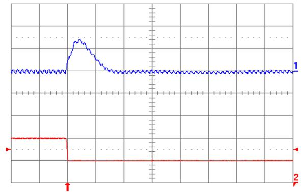
Fig. 1.8V.8: Output voltage response for  $V_{out} = 1.8\text{ V}$  to negative load current step change from 10 A to 5 A with slew rate of  $-5\text{ A}/\mu\text{s}$  at  $V_{in} = 5\text{ V}$ . Top trace: output voltage (100 mV/div.); Bottom trace: load current (5 A/div.).  $C_o = 47\text{ }\mu\text{F}$  ceramic +  $1\text{ }\mu\text{F}$  ceramic. Time scale: 20  $\mu\text{s}$ /div.
