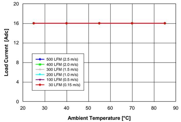
Fig. 1.8V.2: Available load current vs. ambient temperature and airflow rates for  $V_{out} = 1.8\text{ V}$  converter mounted horizontally with  $V_{in} = 5\text{ V}$ , and maximum MOSFET temperature  $\leq 120\text{ }^\circ\text{C}$ .
