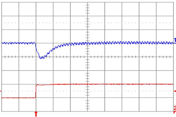
Fig. 1.8V.7: Output voltage response for  $V_{out} = 1.8\text{ V}$  to positive load current step change from 5 A to 10 A with slew rate of  $5\text{ A}/\mu\text{s}$  at  $V_{in} = 5\text{ V}$ . Top trace: output voltage (100 mV/div.); Bottom trace: load current (5 A/div.).  $C_o = 47\text{ }\mu\text{F}$  ceramic +  $1\text{ }\mu\text{F}$  ceramic. Time scale: 20  $\mu\text{s}$ /div.
