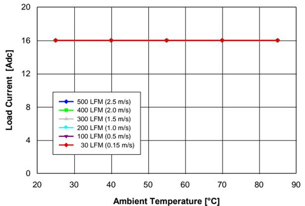
Fig. 0.7525V.2: Available load current vs. ambient temperature and airflow rates for  $V_{out} = 0.7525\text{ V}$  converter mounted horizontally with  $V_{in} = 5\text{ V}$ , and maximum MOSFET temperature  $\leq 120\text{ }^\circ\text{C}$ .
