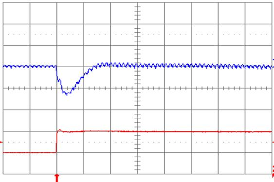
Fig. 1.5V.7: Output voltage response for  $V_{out} = 1.5\text{ V}$  to positive load current step change from 5 A to 10 A with slew rate of  $5\text{ A}/\mu\text{s}$  at  $V_{in} = 5\text{ V}$ . Top trace: output voltage (100 mV/div.); Bottom trace: load current (5 A/div.).  $C_o = 47\text{ }\mu\text{F}$  ceramic +  $1\text{ }\mu\text{F}$  ceramic. Time scale: 20  $\mu\text{s}$ /div.
