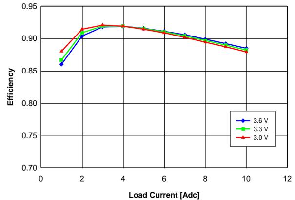
Fig. 1.2V.4: Efficiency vs. load current and input voltage for  $V_{out} = 1.2\text{ V}$  converter mounted vertically with air flowing at a rate of 200 LFM (1 m/s) and  $T_a = 25\text{ }^{\circ}\text{C}$ .
