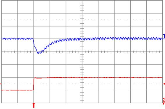
Fig. 2.0V.7: Output voltage response for  $V_{out} = 2.0\text{ V}$  to positive load current step change from 5 A to 10 A with slew rate of  $5\text{ A}/\mu\text{s}$  at  $V_{in} = 5\text{ V}$ . Top trace: output voltage (100 mV/div.); Bottom trace: load current (5 A/div.).  $C_o = 47\text{ }\mu\text{F}$  ceramic +  $1\text{ }\mu\text{F}$  ceramic. Time scale:  $20\text{ }\mu\text{s}/\text{div}$ .
