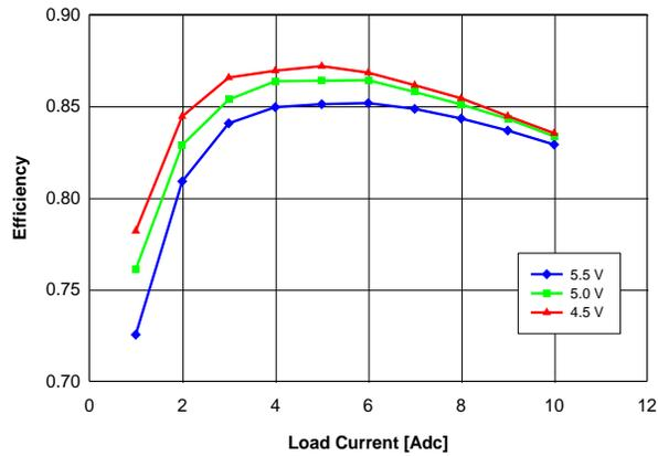
Fig. 0.7525V.3: Efficiency vs. load current and input voltage for  $V_{out} = 0.7525\text{ V}$  converter mounted vertically with air flowing at a rate of 200 LFM (1 m/s) and  $T_a = 25\text{ }^\circ\text{C}$ .
