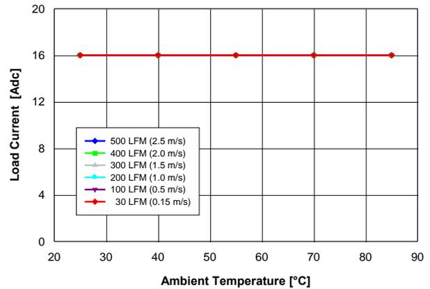
Fig. 1.0V.2: Available load current vs. ambient temperature and airflow rates for  $V_{out} = 1.0\text{ V}$  converter mounted horizontally with  $V_{in} = 5\text{ V}$ , and maximum MOSFET temperature  $\leq 120\text{ }^\circ\text{C}$ .
