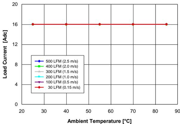
Fig. 0.7525V.1: Available load current vs. ambient temperature and airflow rates for  $V_{out} = 0.7525\text{ V}$  converter mounted vertically with  $V_{in} = 5\text{ V}$ , and maximum MOSFET temperature  $\leq 120\text{ }^\circ\text{C}$ .
