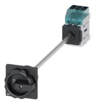
Load disconnector 3LD3, lu 25 A Main switch 3-pole Rated operating capacity at AC-23 A at 400V 9.0kW floor mounting Basic switch with door coupling Central hole mounting 22.5mm Rotating drive black 66 x 66 mm
