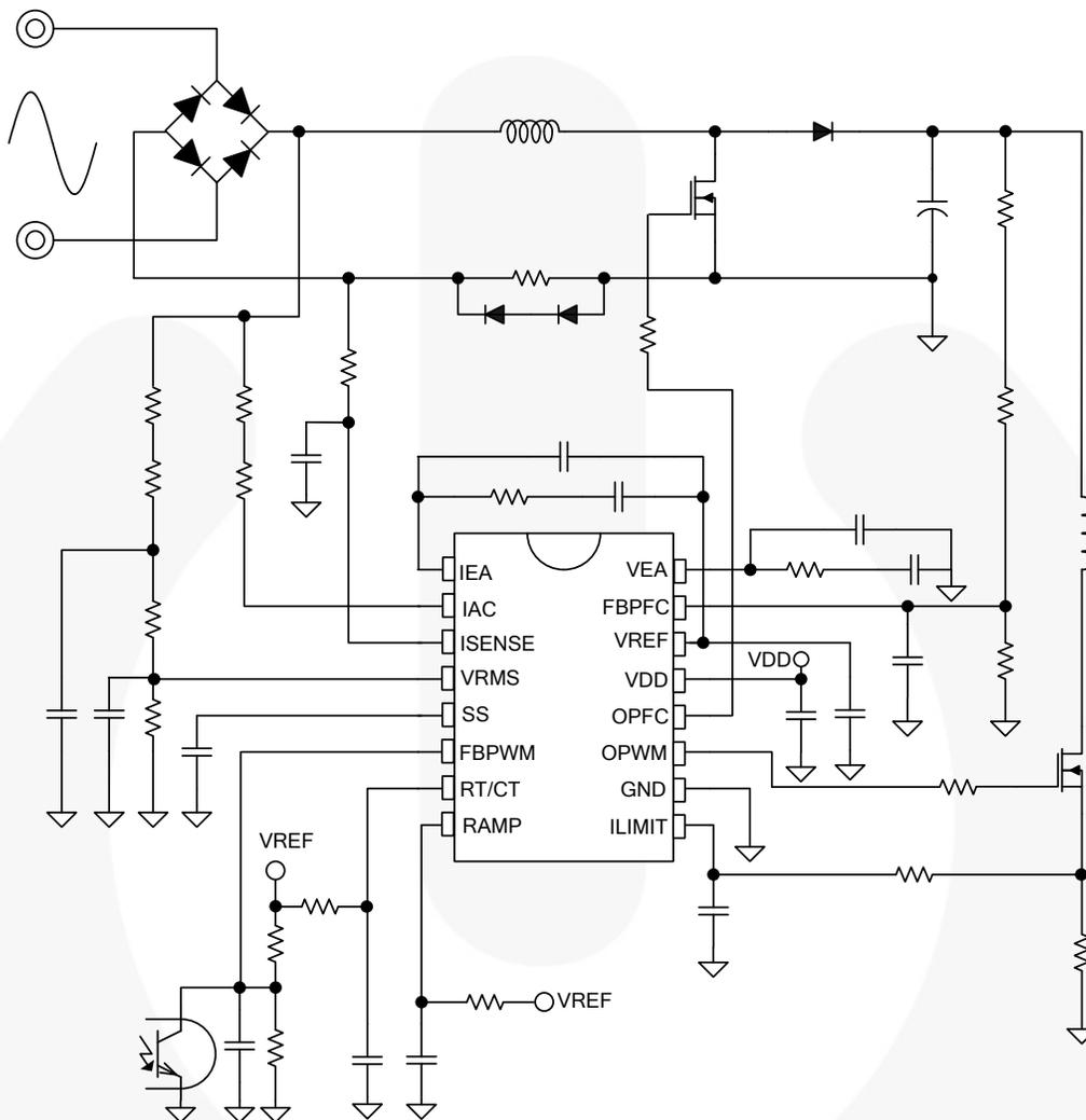
Figure 2. Typical Application, Voltage Mode
