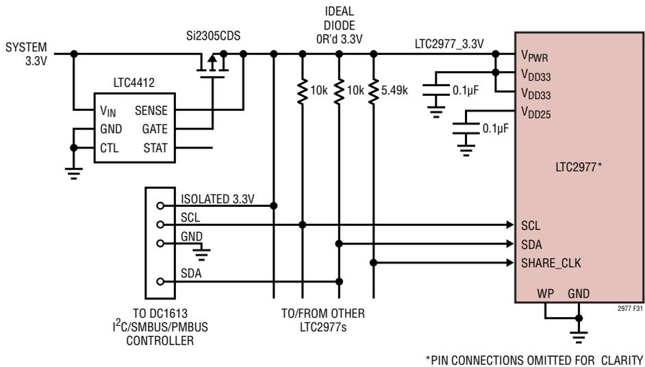
NOTE: DC1613 CONTROLLER I<sup>2</sup>C CONNECTIONS ARE OPTO-ISOLATED
