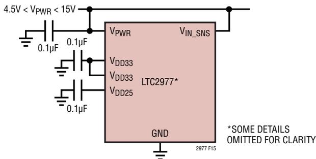
Figure 15. Powering LT2977 Directly from an Intermediate Bus
