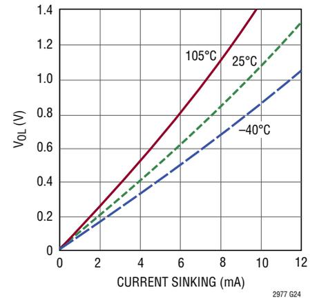
**V<sub>OUT\_EN[7:4]</sub> V<sub>OL</sub> vs Current**
