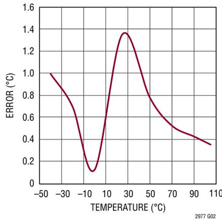
**ADC Total Unadjusted Error vs Temperature**
