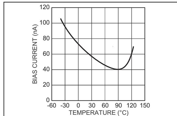
**FIGURE 2-6:** Feedback Input Bias Current vs. Temperature.
