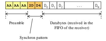
The first 3 bytes compose a 24 bit length '01' pattern to let enough time for the clock recovery of the receiver to lock. The next two bytes compose a 16 bit synchron pattern which is essential for the receiver's FIFO to find the byte synchron in the received bit stream. The synchron patters is followed by the payload. The first byte transmitted after the synchron pattern ( $D_0$  in the picture above) will be the first received byte in the FIFO.
