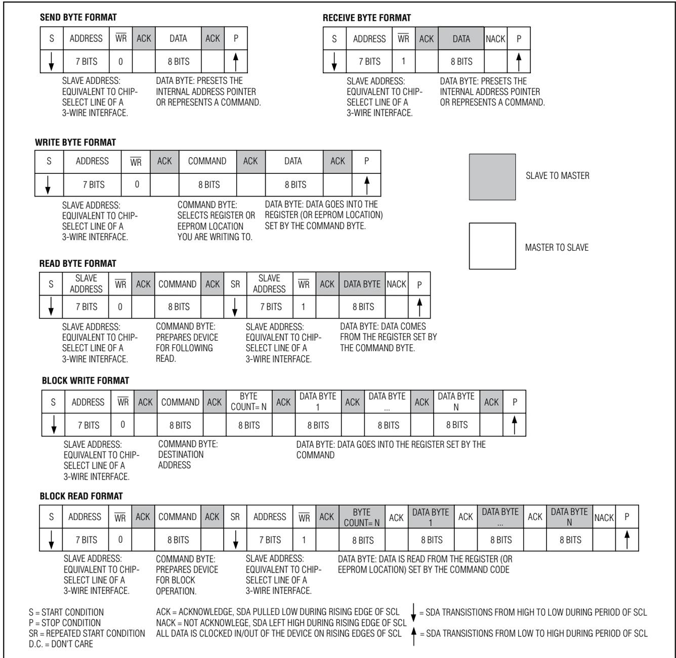
Figure 12. I<sup>2</sup>C/SMBus Protocols
