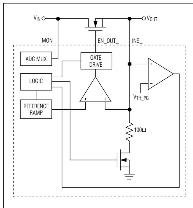
Figure 5. Closed-Loop Tracking
