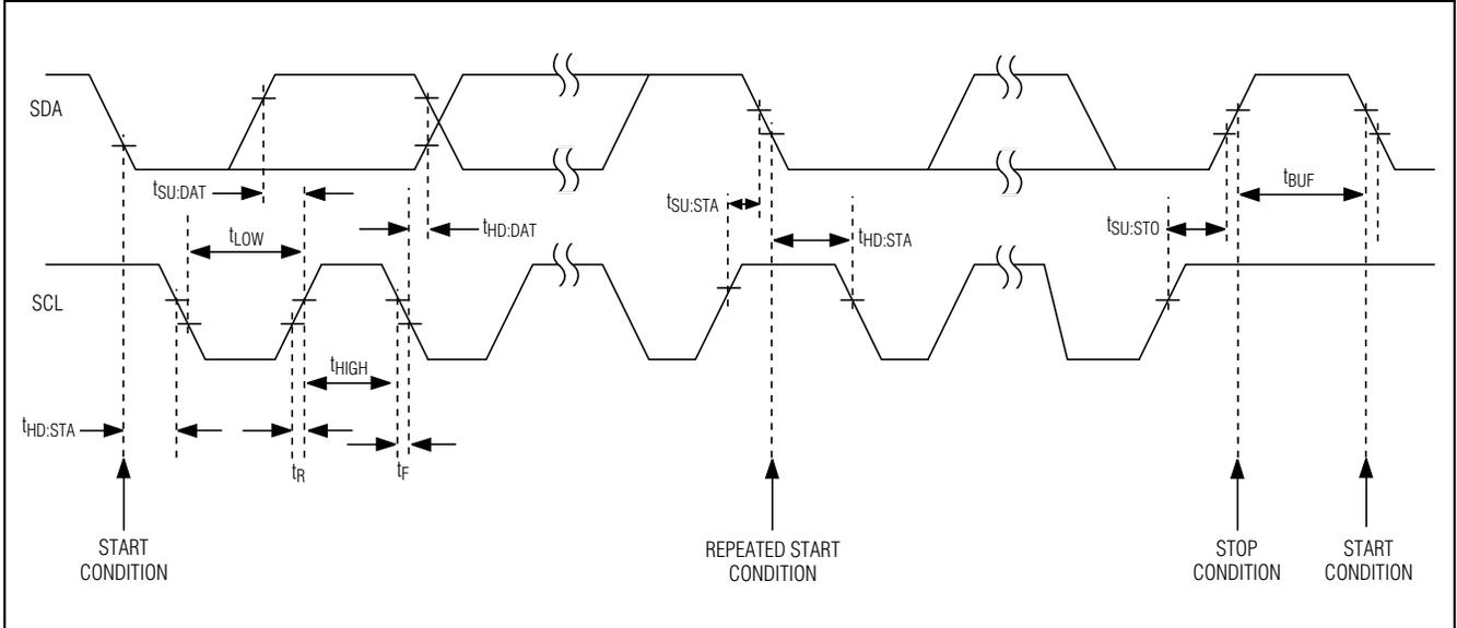
Figure 1. I<sup>2</sup>C/SMBus Timing Diagram
