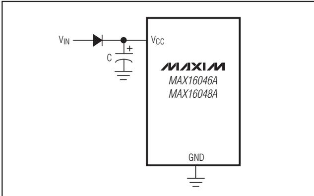
Figure 18. Power Circuit for Shutdown During Fault Conditions
